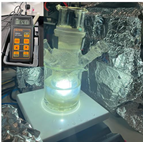
Figure 18: Internally illuminated photoreactor heating up after 60 min of reaction.
