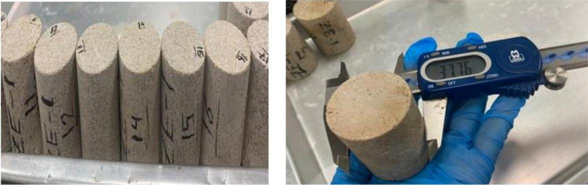
Figure 11: Core Samples Measurements
