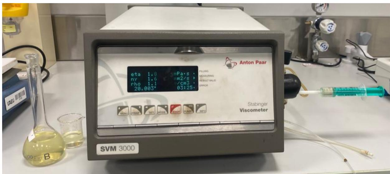
Figure 20: Anton Paar Stabinger Viscometer Device Used for Viscosity and Density Measurements
