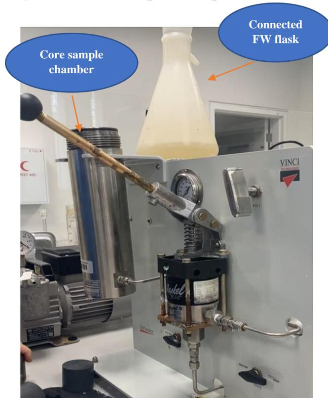
Figure 13: Core Saturation Apparatus
