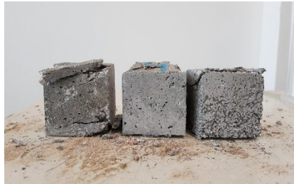
Figure 17: Tested cubes for compressive strength
