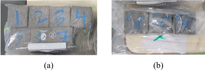
Figure 15: Post-carbonation curing techniques. (a) Sealed subsequent hydration and (b) water-sprayed hydration
