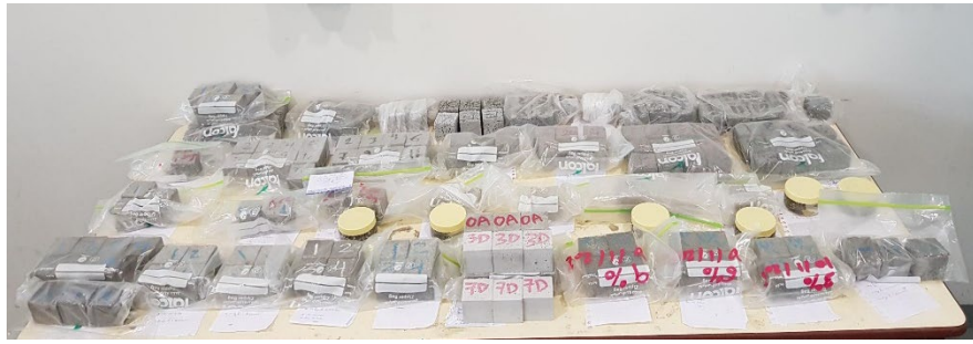
Figure 11: Concrete mixes after casting and curing
