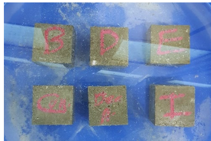
Figure 19: Immersed cubes for water absorption
