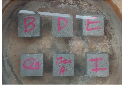
Figure 20: Boiled samples for permeable voids pore volume
