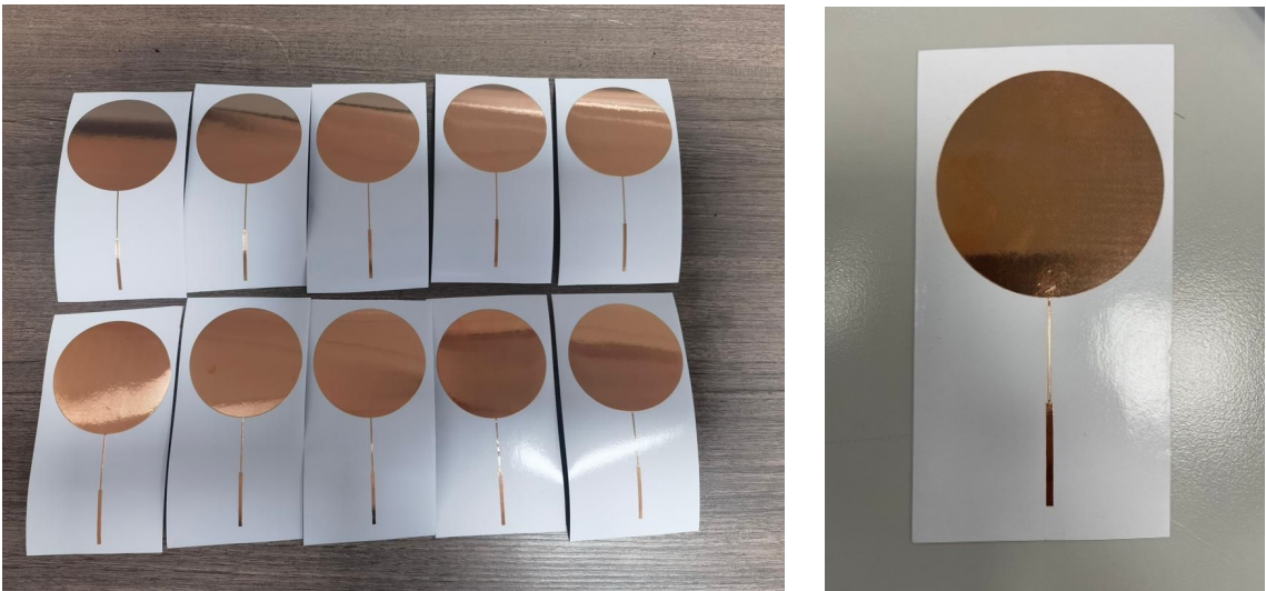
Figure 2.3: Circular edge-fed patch antenna final product
