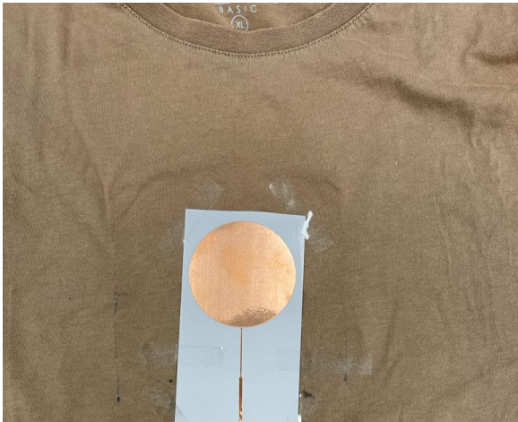
Figure 3.8: Circular patch antenna with stretchable textile substrate
