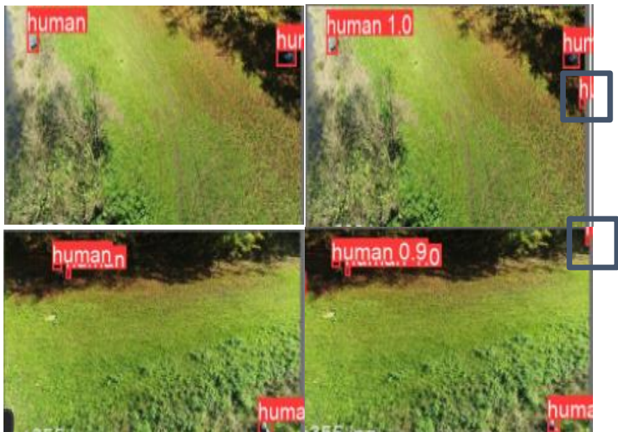
Figure 15: False detections of YOLO-v5 model (shadows, dark areas)
