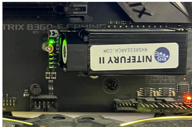
Figure 3.22: The FPGA connected to the PC through the PCIe enabled M.2 slot
