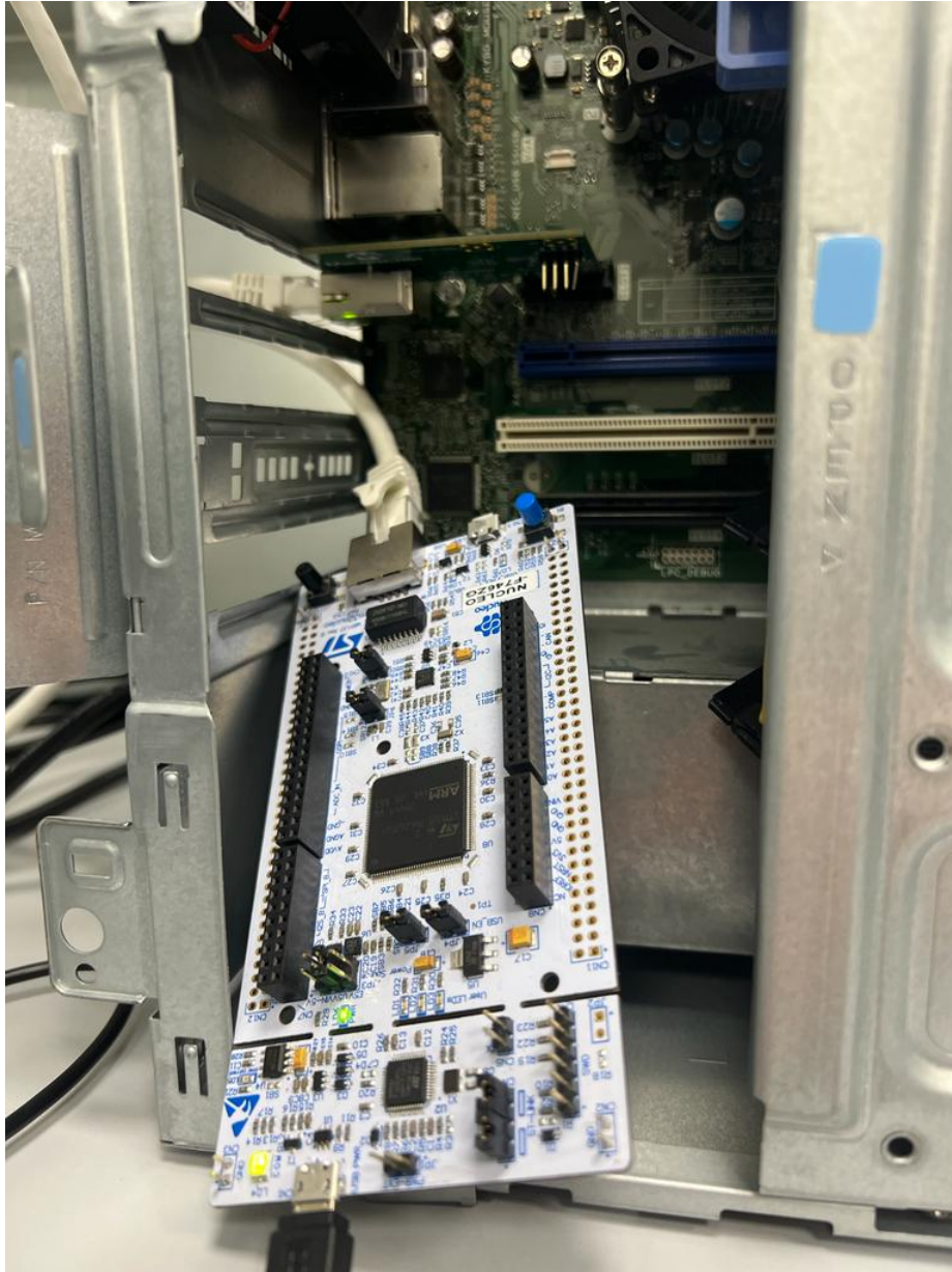
Figure 3.31: The microcontroller and cPCI backplane (represented by a PC) data transfer test setup
