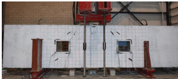
Figure 2.2: A typical deep beam with cutouts during testing [34]
