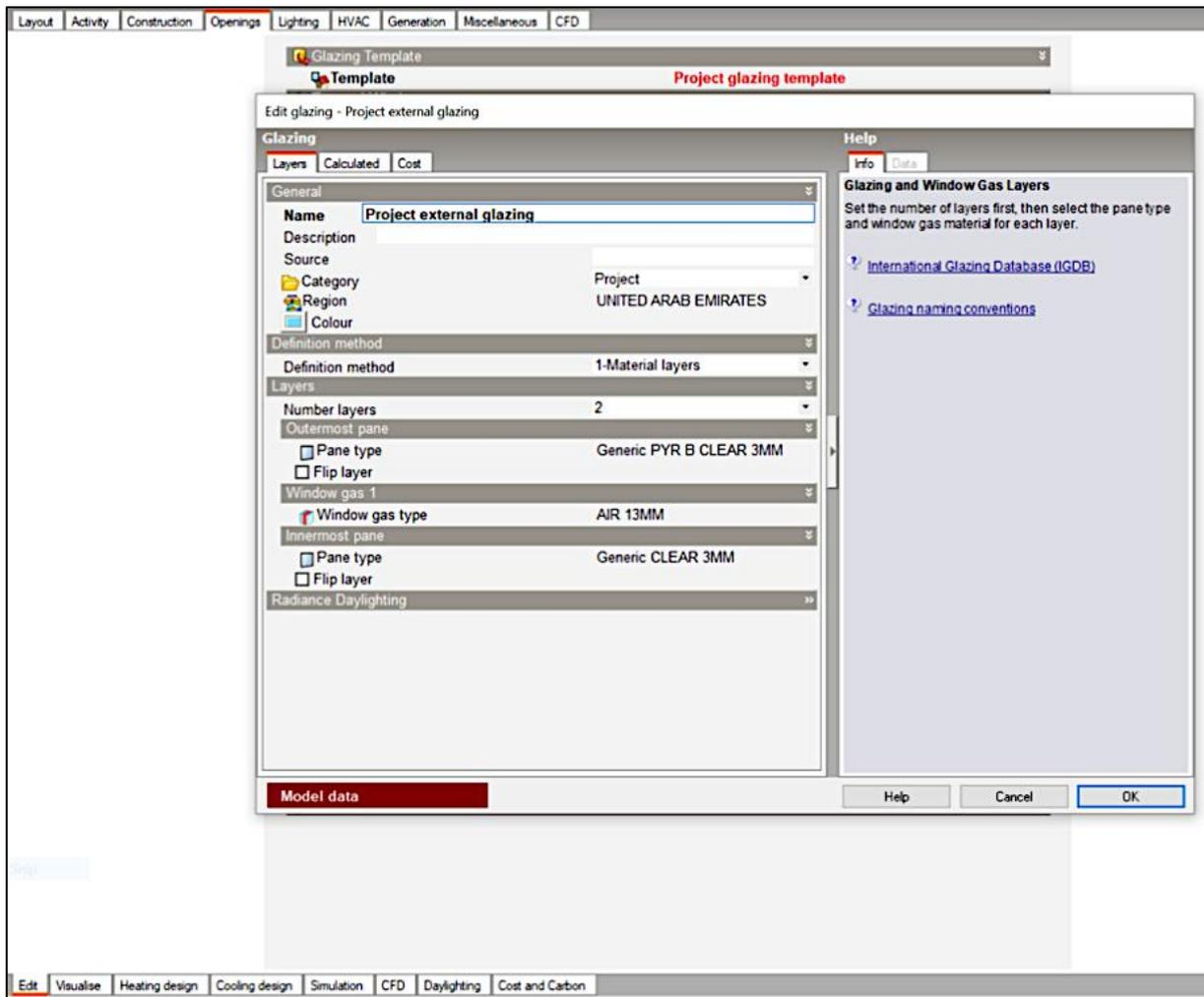
Figure C 9: External Glazing Details
