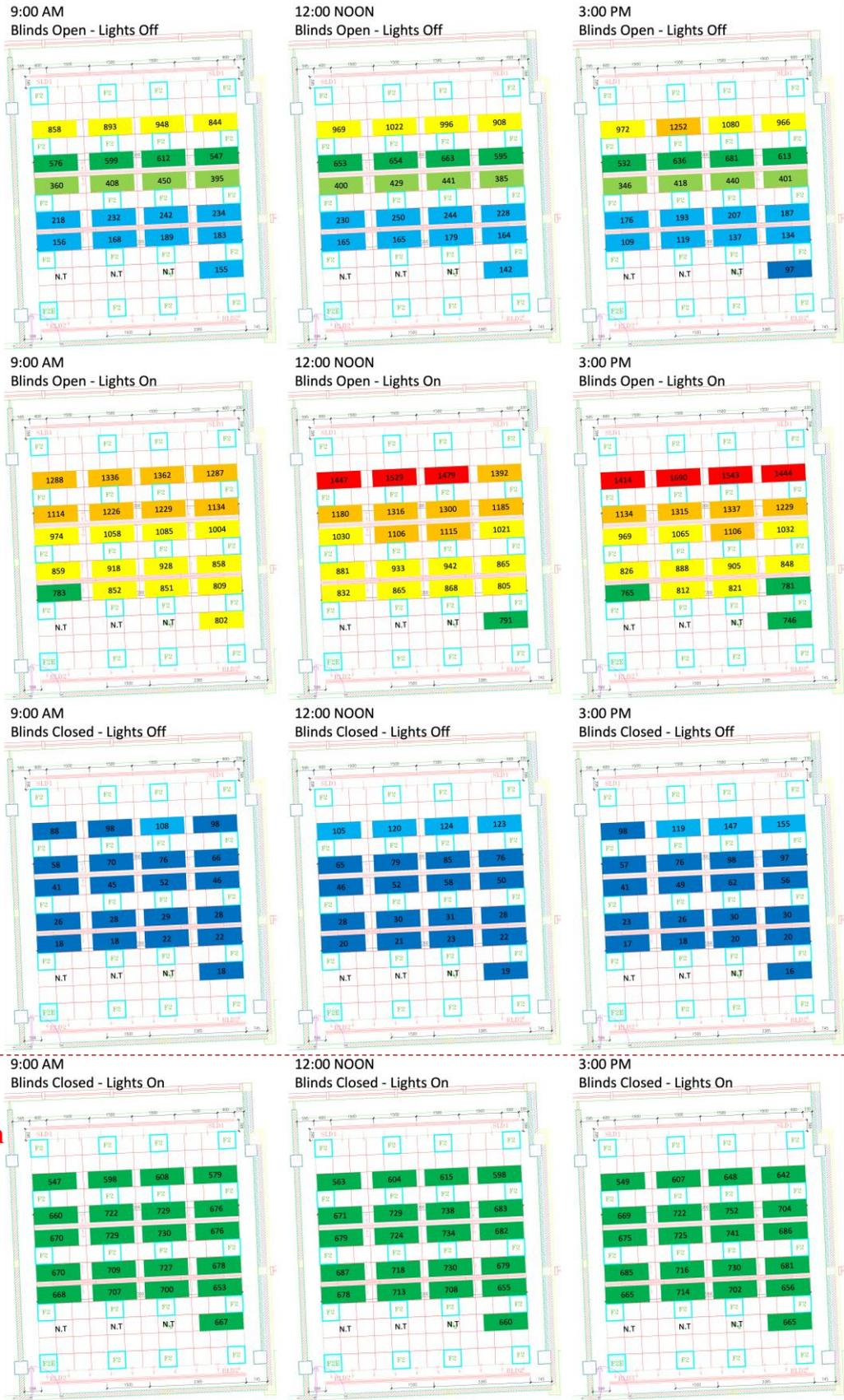
Figure 45: Lighting Levels Measurements for Classroom 1037 (First Floor)
