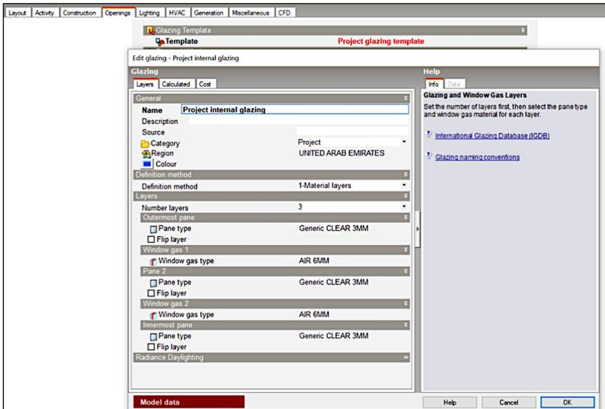
Figure C 10: Internal Glazing Details
