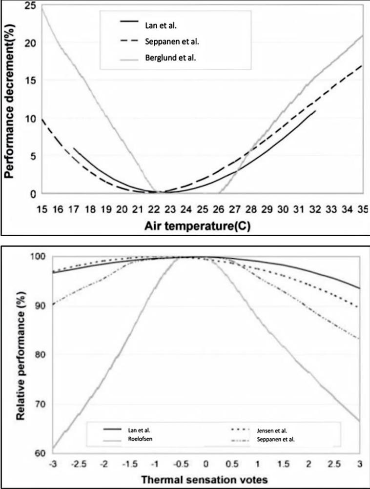
Figure 8: Comparison of the Relationship Between Air Temperatures (Top) and Thermal Sensation Votes (Down) with Relative Performance Developed in Three Studies in Office Workers. Source: (Chatzidiakou et al., 2014)
