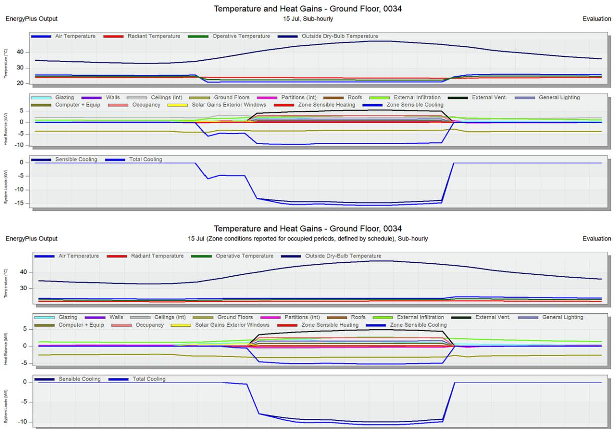
Figure 47: Cooling Load Graphs from DesignBuilder Software for Classroom 0034
