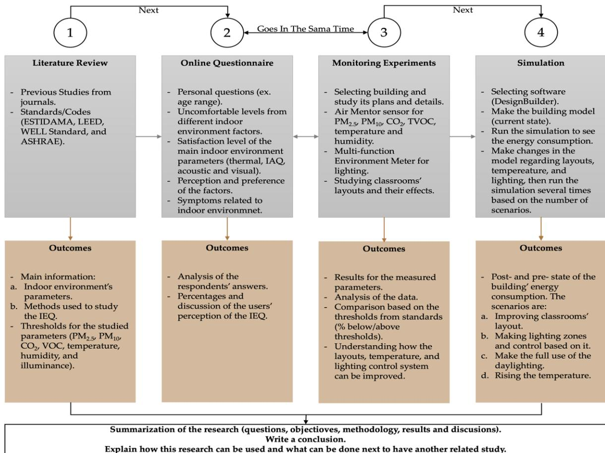
Figure 11: Research Procedure with Four Main Methods
