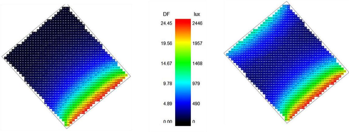
Figure 52: Current State of Lux Distribution in classroom 0034 (Left) and After Opening the Side Window Through the Corridor (Right)
