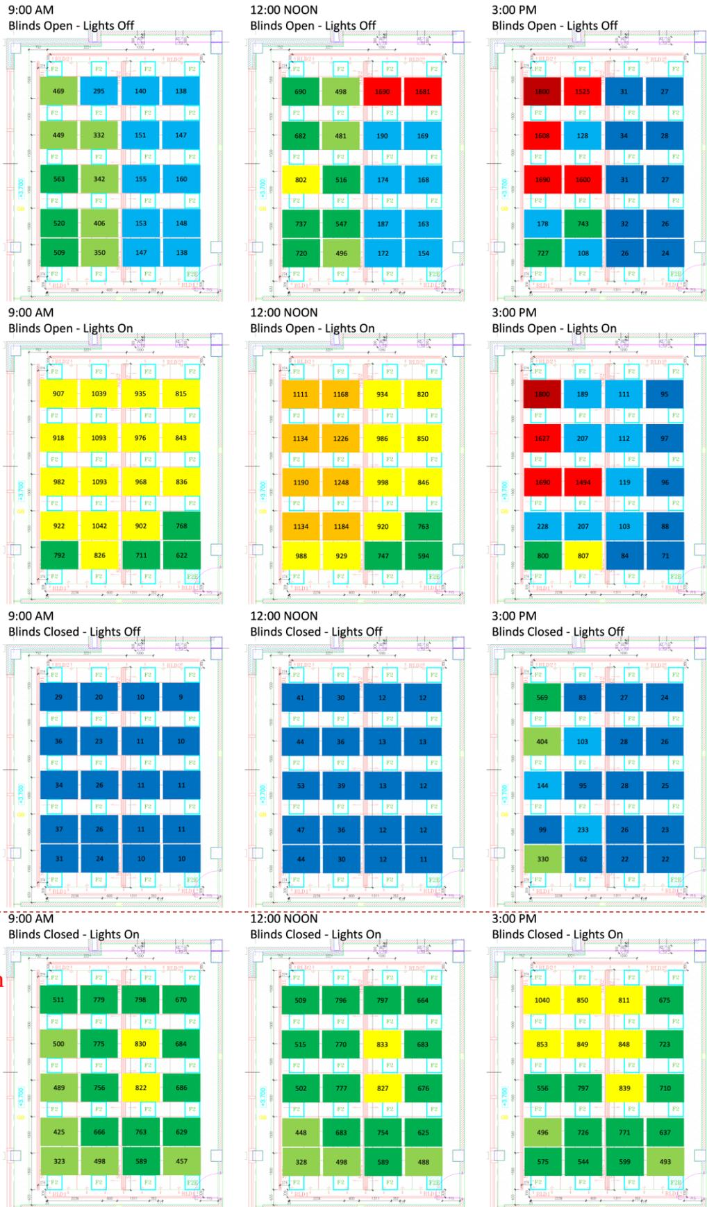
Figure 39: Lighting Levels Measurements for Classroom 1015 (First Floor)
