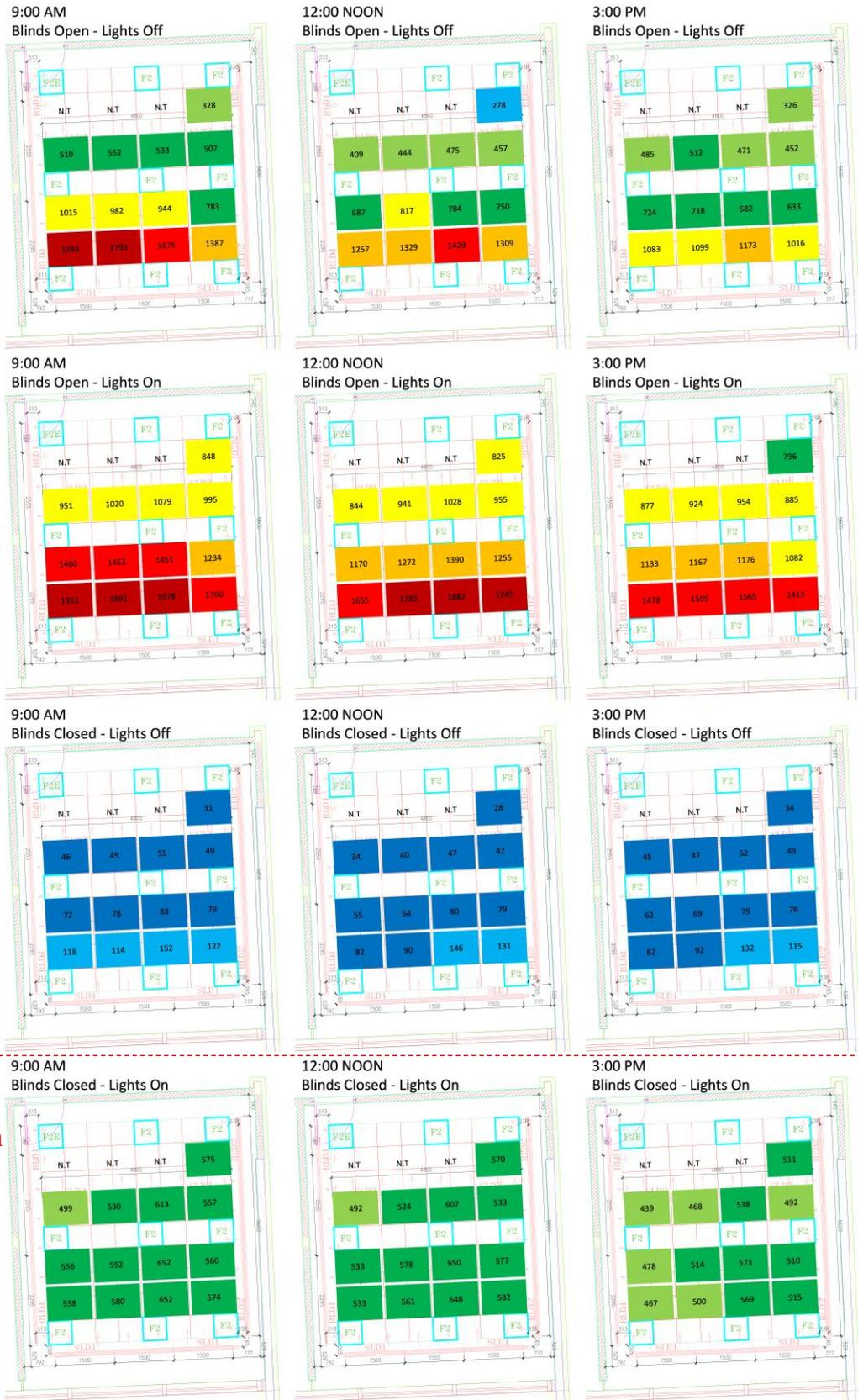
Figure 42: Lighting Levels Measurements for Classroom 1036 (First Floor)
