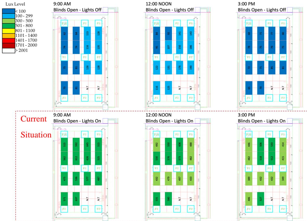
Figure 36: Lighting Levels Measurements for Classroom 1012 (First Floor)
