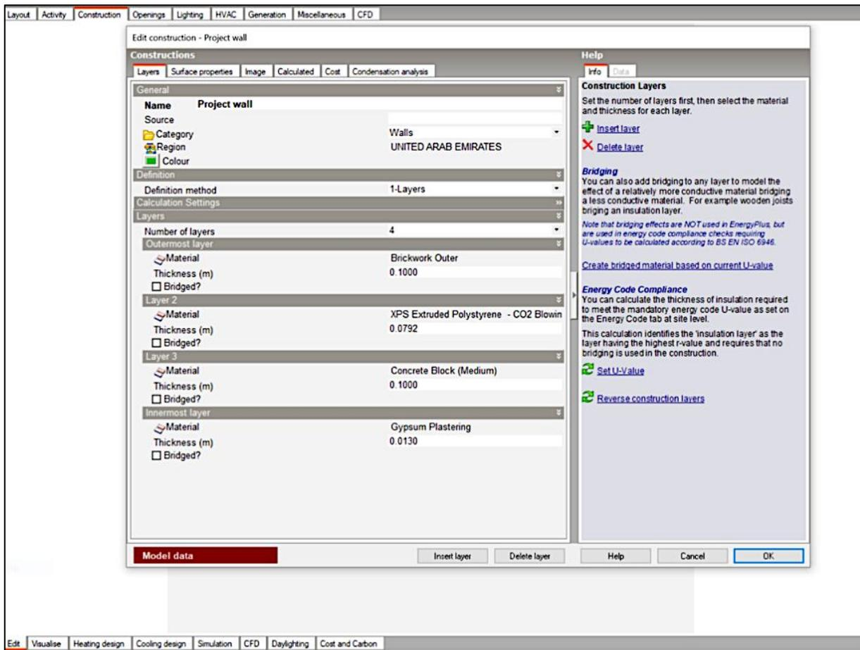
Figure C 5: External Walls Construction Details
