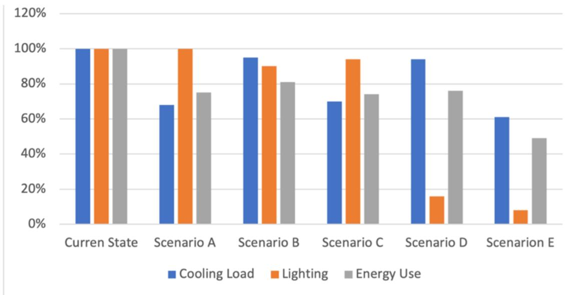
Figure 53: The Reduction in Cooling Load, Lighting, and Energy Use of All the Scenarios
