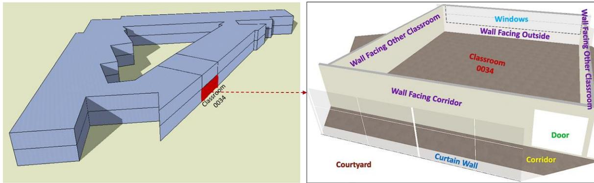
Figure 16: 3D Model and Classroom 0034 Created in DesignBuilder Software
