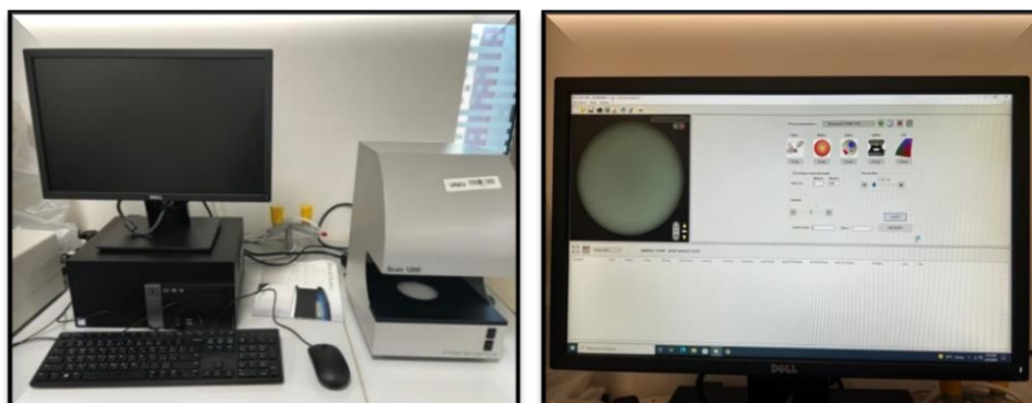
Figure 29: Interscience Scan 1200 device for viable probiotic cells count
