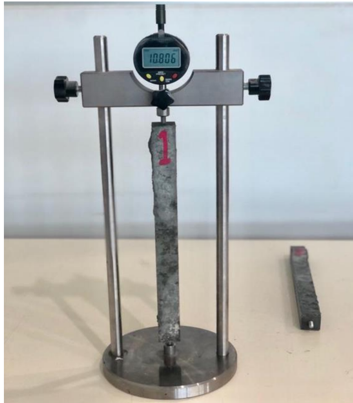
Figure 35: Drying shrinkage test setup.
