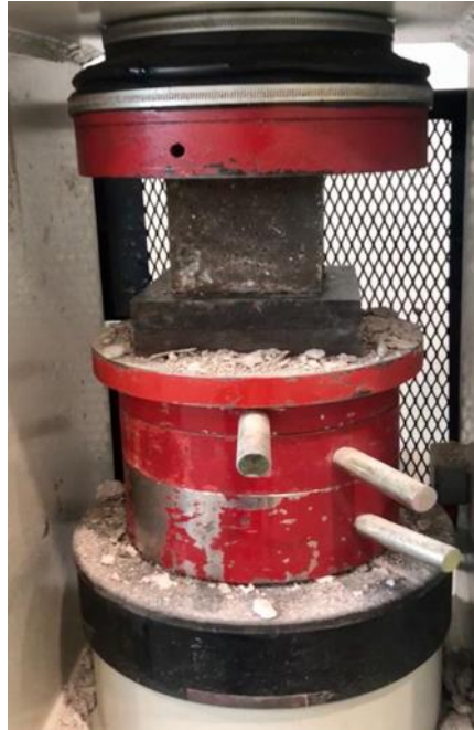
Figure 32: Compressive strength test.
