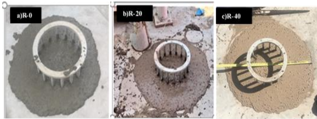
Figure 51: J-ring test for SCC mixtures.
