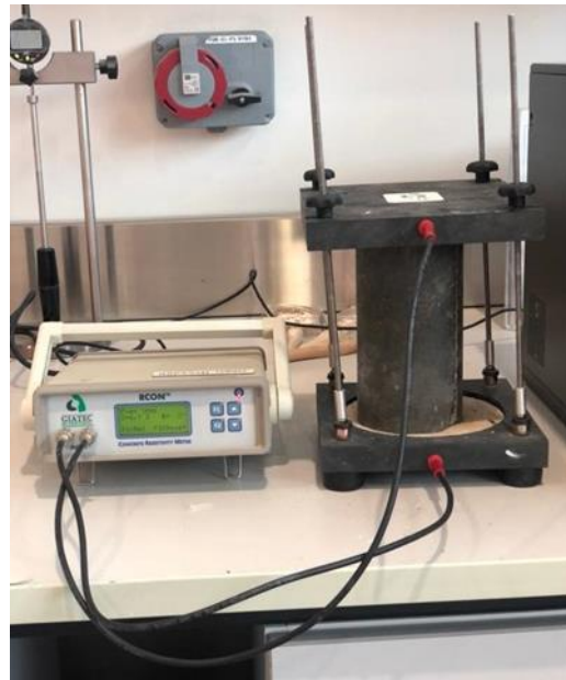
Figure 33: Electrical resistivity test setup.
