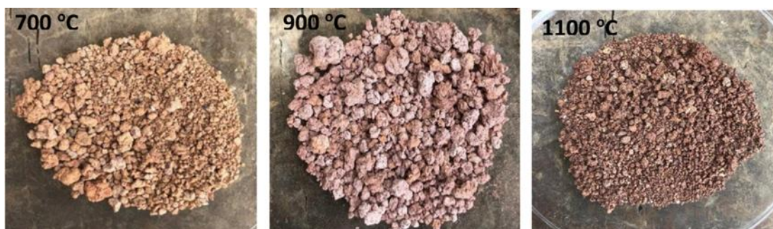
Figure 24: Incinerated SSA particles before grinding.
