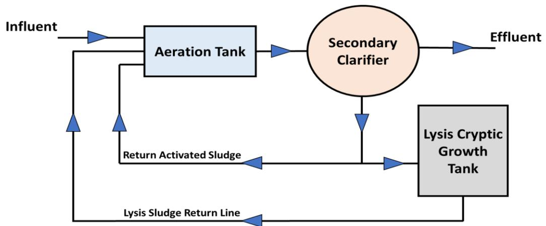
Figure 9: Lysis Cryptic Growth Technique (Guo et al., 2013)
