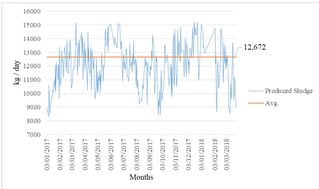
Figure 18: Produced Dewatered Sludge at Al Saad WWTP
