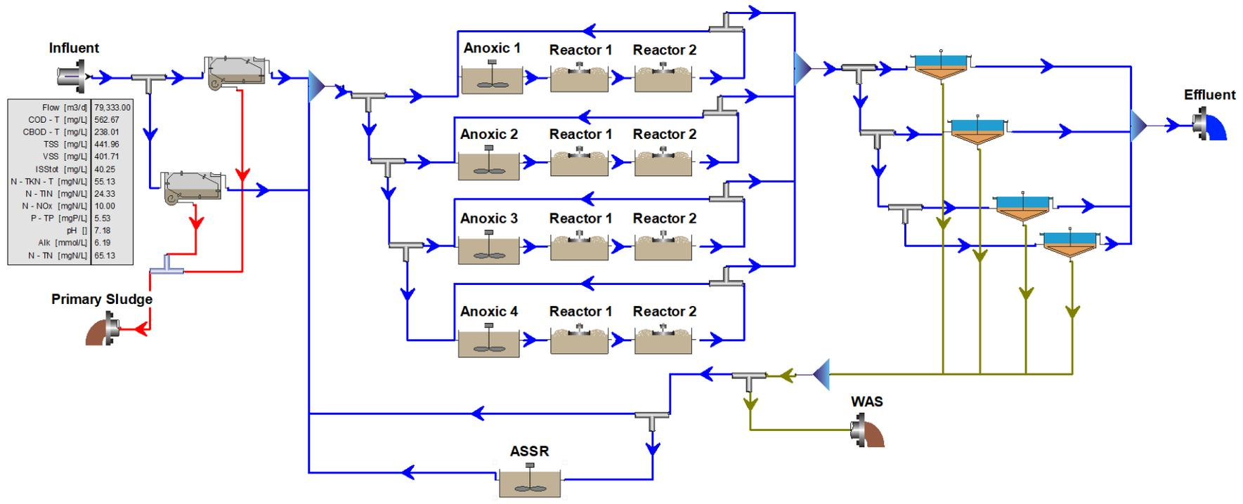
Figure 24: Model layout of Al-Saad WWTP with ASSR Process
