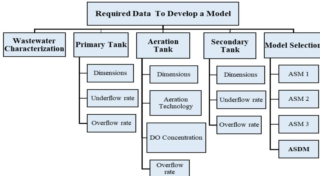
Figure 15: Required Data to Build a Model
