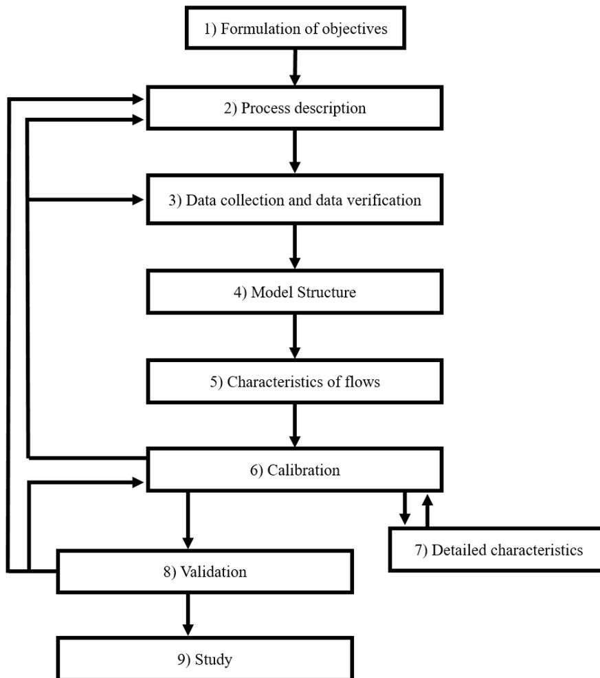
Figure 3: STOWA Model Calibration Procedures (Sin et al., 2005)
