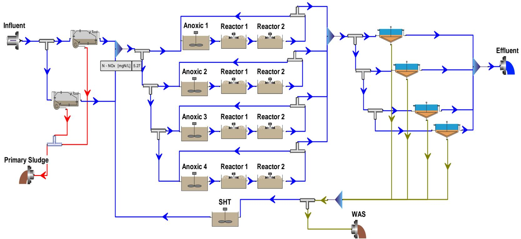
Figure 23: Model layout of Al-Saad WWTP with OSA Process
