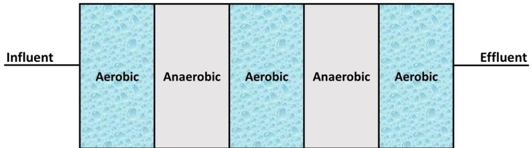
Figure 11: Repeatedly Coupling of Aerobic/Anaerobic Process (Guo et al., 2013)
