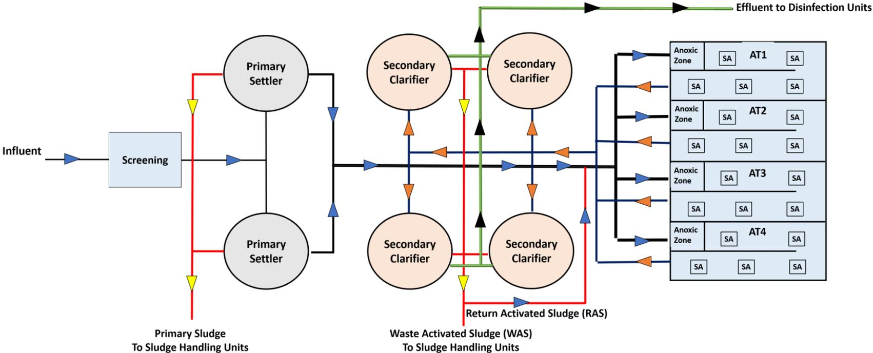
Figure A1: Al-Saad WWTP Schematic Diagram
