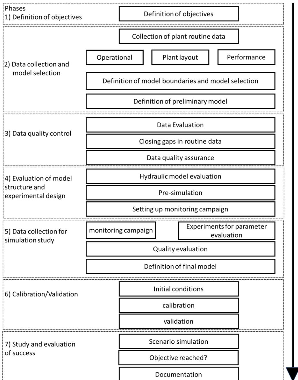
Figure 4: HSG Guidelines for Model Calibration (Sin et al., 2005)
