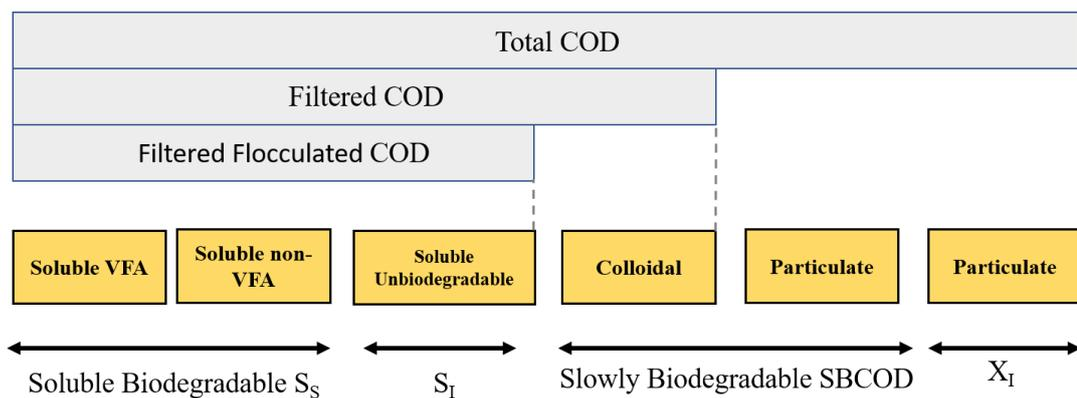
Figure 6: Physical Separation for Determination of COD Fractions (Melcer, 2003)
