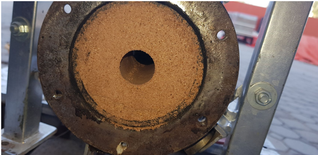
Figure 17: Propellant grains inside the combustion chamber.
