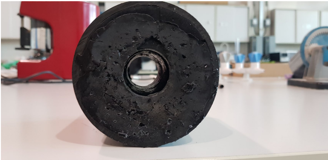
Figure 19: The propellant after being cooled and ready for the burning test.
