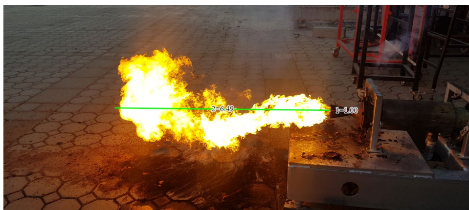
Figure 45: Representation of measuring methodology for the PW flame length at an oxidizer volume flow rate of 130 lpm. Where 6.49 equals 100.4 cm.
