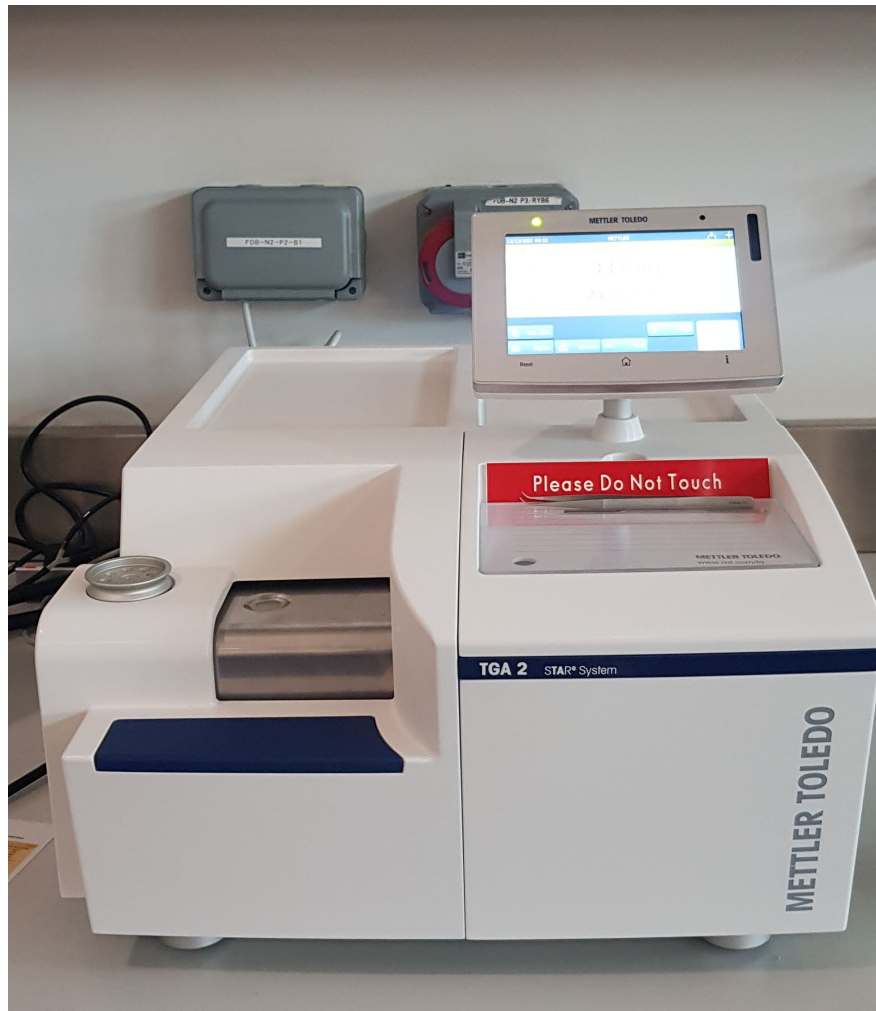
Figure 22: Device used for GTA test from METTLER TOLEDO.
