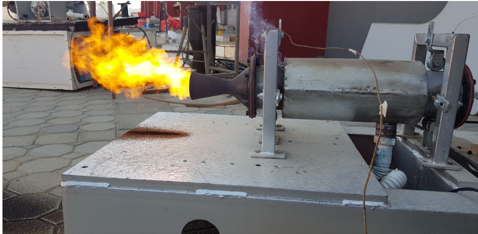
Figure 13: Rocket testing facility with cooling system.
