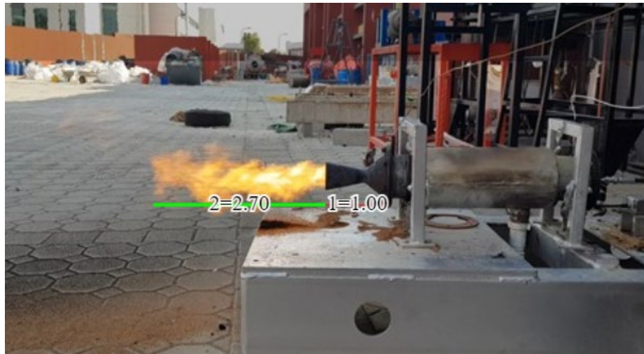
Figure 46: Flame length of Date Stone propellant at 130 lpm where 2.7 equals 41.8 cm.
