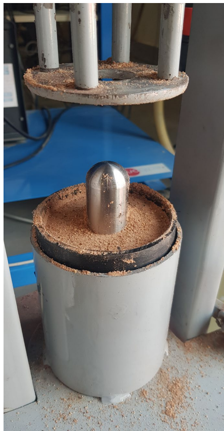
Figure 16: Propellant grains after compression process.
