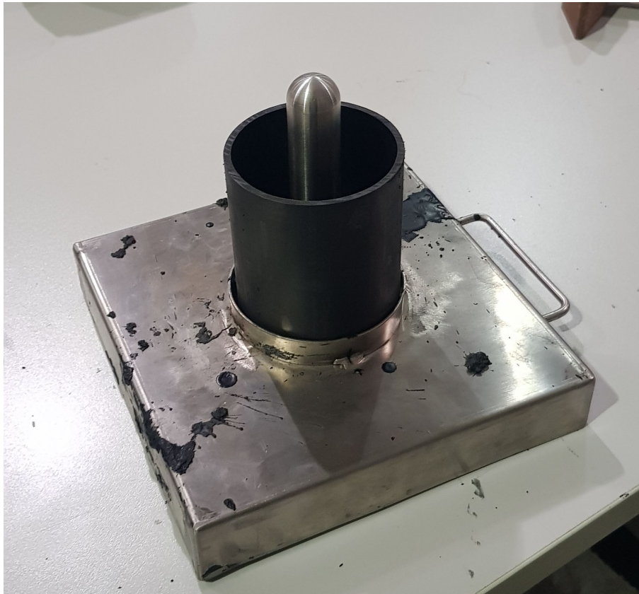
Figure 18: The stand and mold for PW-based propellant.
