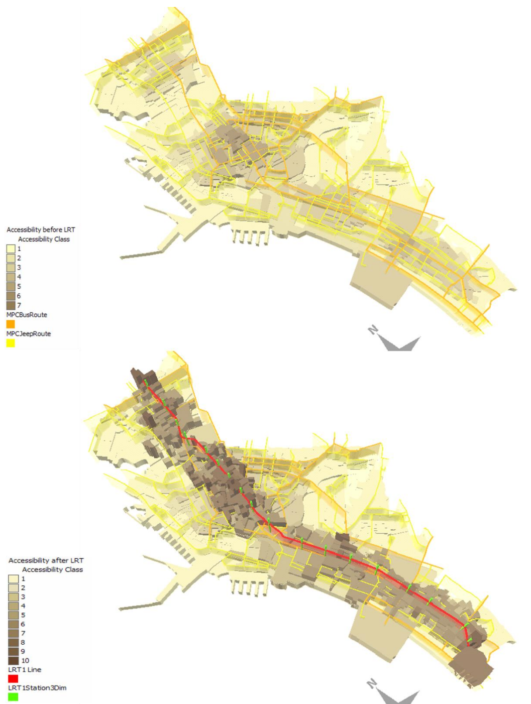
Figure 15: The accessibility GIS analysis results, highlighting the changes in two scenarios; before (top) and after LRT1 (bottom). Adapted from (Raguz, 2010)
