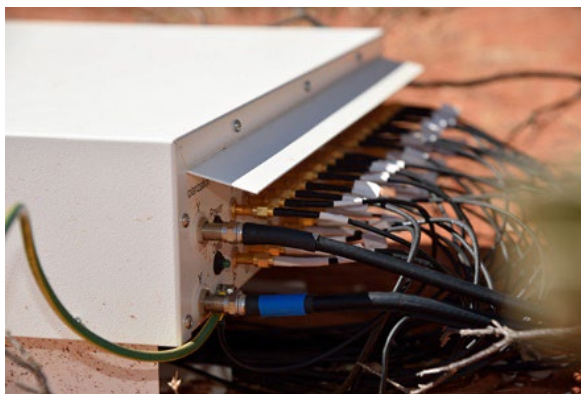
Figure 18: Beamformer connected to 16 antennas
