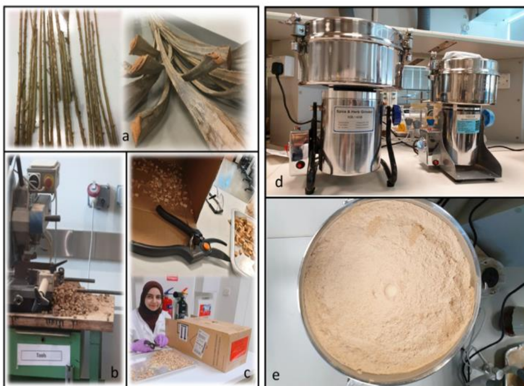
Figure 17: Date Palm Rachis preparations and size reduction. (a) rachis collection, (b) rachis shredding, (c) further chopping using a lopper, (d) size reduction by grinder, and (e) ground sample ready for sieving.
