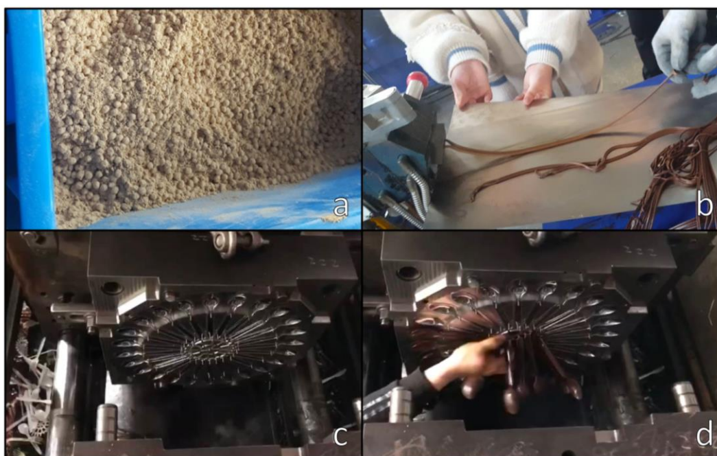
Figure 35: Industrial fabrication of cutlery from 30 wt% DPR-PLA composite. (a) mixed PLA and DPR, (b) melt mixing extrusion, (c) two plates with mold cavity of spoons shape ready for injection molding, and (d) spoons collection after the two plates separation of the mold.
