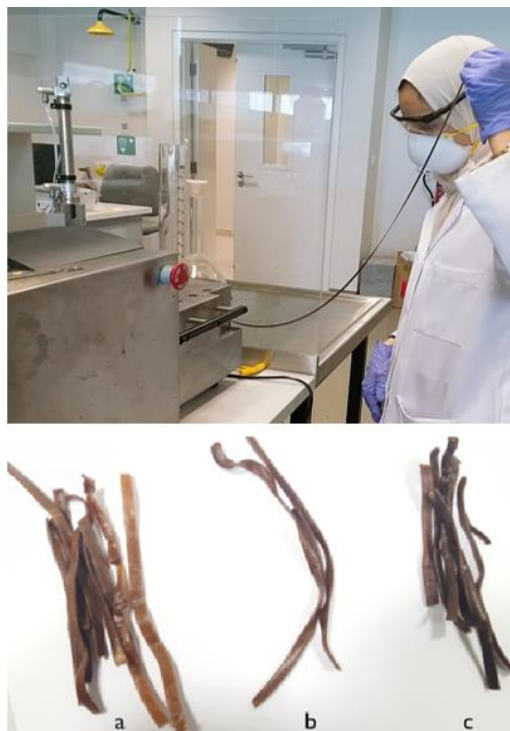
Figure 19: 30% DPR-PLA composites fabrication using two screw extruders with different mixing times. (a) 7 min PLA, 3 min biomass, (b) 5 min PLA, 5 min biomass, and (c) 3 min PLA, 7 min biomass.
