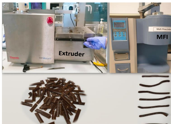
Figure 23: Extruded DPR-PLA composite was broken into small pieces to be inserted in the barrel of the MFI machine.
