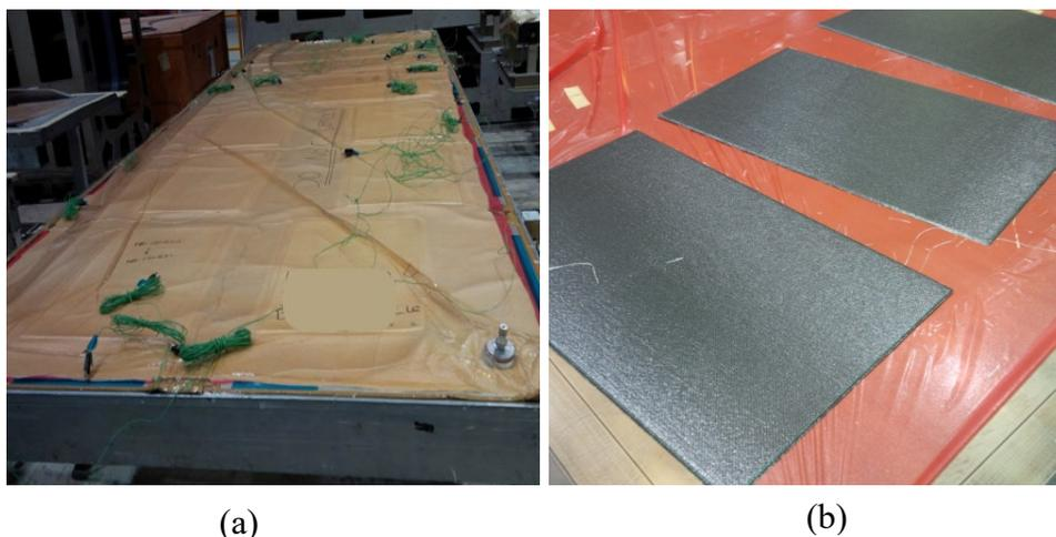
Figure 23: Debugging of test panels. (a) Tool after being removed from the autoclave
