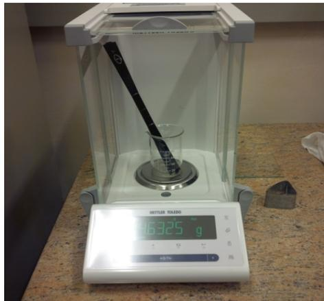
Figure 37: Sensitive scale with 4 decimal place resolution
