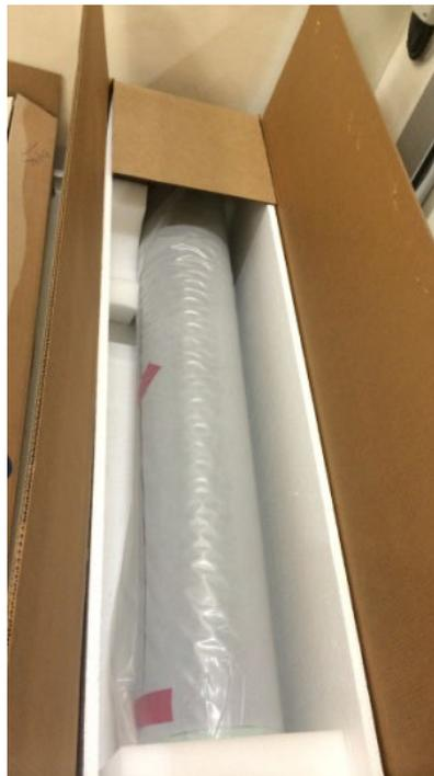
Figure 14: Thawing of the pre-impregnated carbon roll
