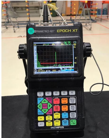
Figure 26: Epoch XT Ultrasonic Flaw Detector
