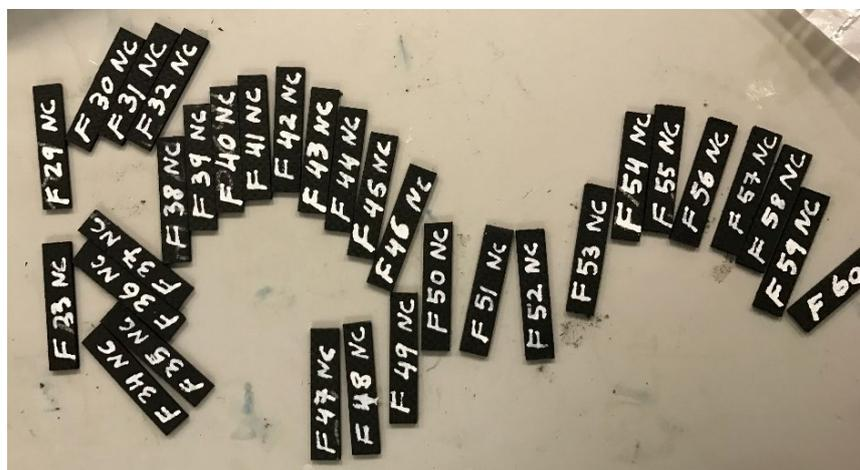
Figure 42: Flexural test samples
