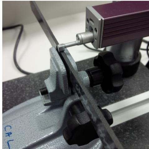
Figure 31: Mitutoyo Surface Roughness Tester SJ 301
