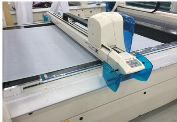
Figure 15: LECTRA ply cutting machine
