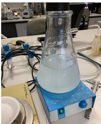
Figure 8: Brine mixing apparatus
