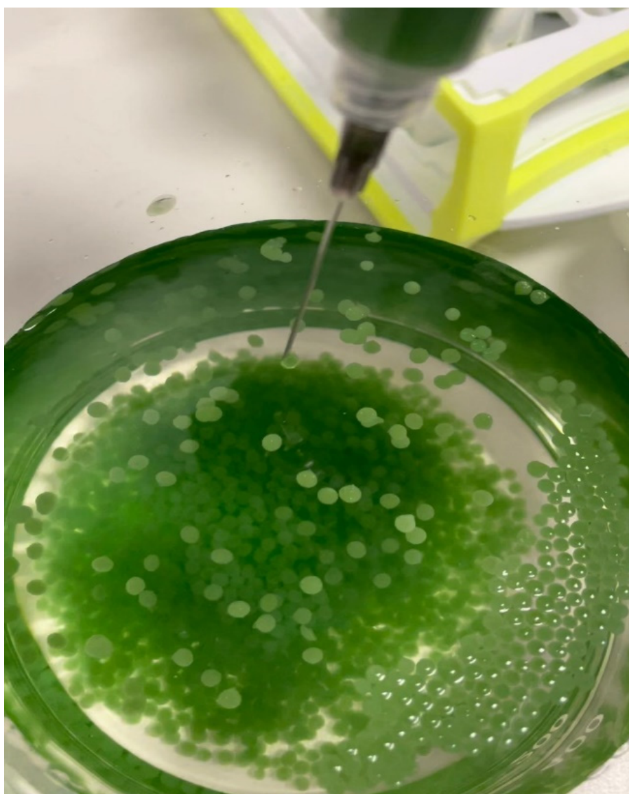
Figure 26: Preparation of immobilized algae beads with alginate.
