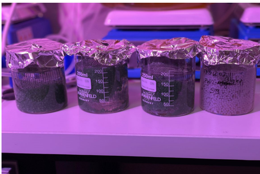
Figure 27: Treatment of PW2 with algae immobilized in alginate beads
