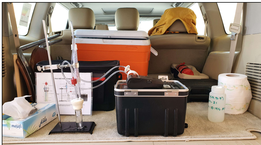
Figure 6: Configuration of the ^{222}\text{Rn} measurement in-situ cabin and the Rad7 instrument
