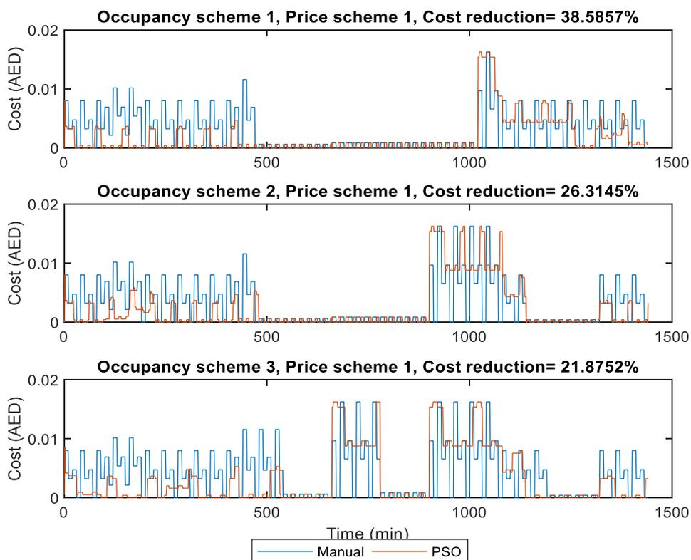
Figure 19: Manual controller cost vs PSO cost for price scheme 1
