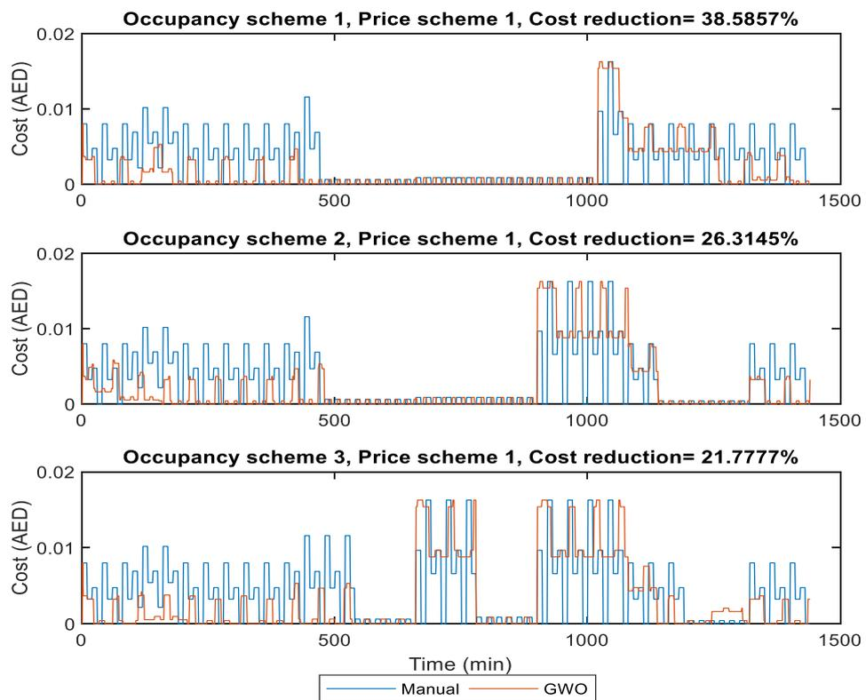
Figure 25: Manual controller cost vs GWO cost for price scheme 1
