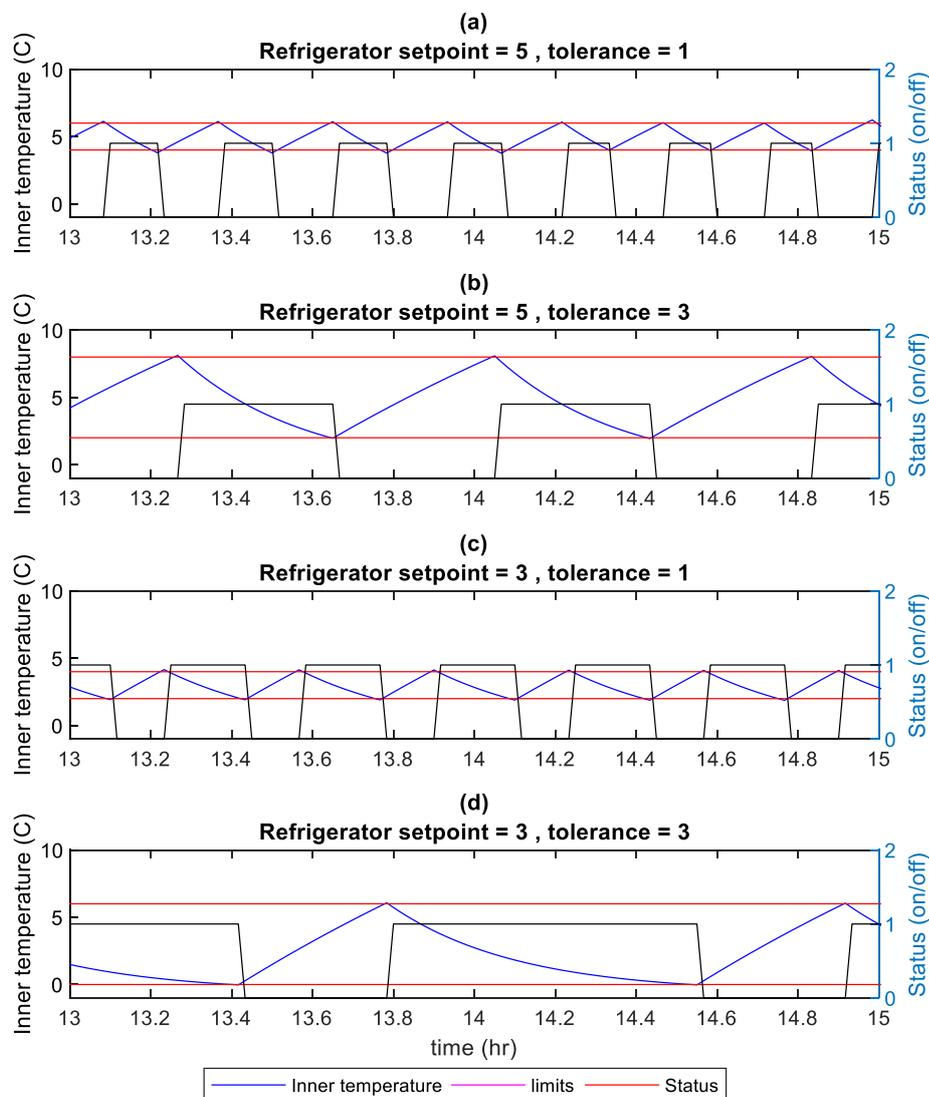
Figure 13: Refrigerator controller output
