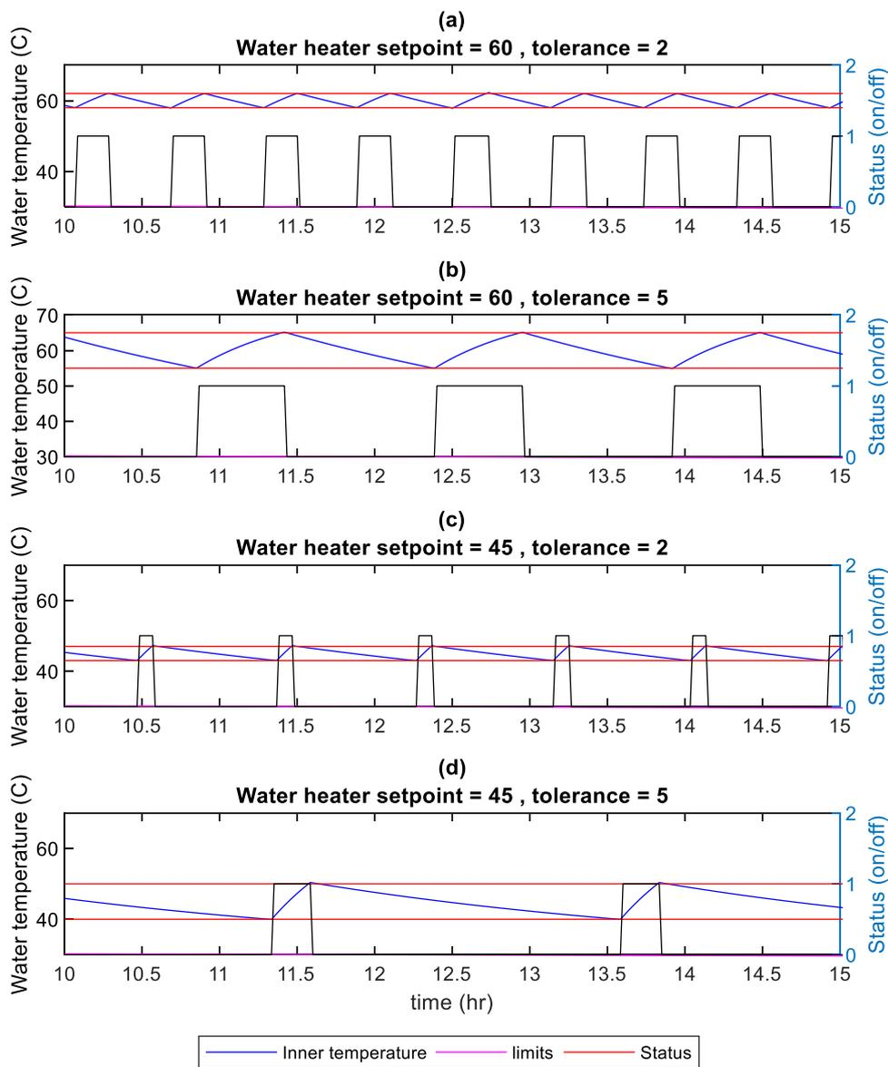
Figure 14: Water heater controller output
