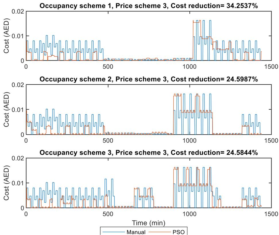
Figure 21: Manual controller cost vs PSO cost for price scheme 3
