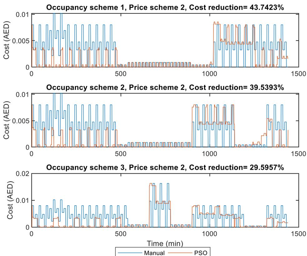
Figure 20: Manual controller cost vs PSO cost for price scheme 2
