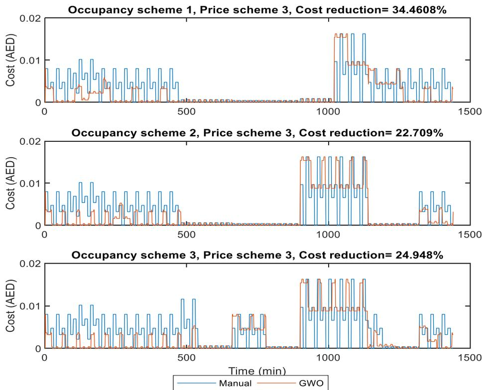
Figure 27: Manual controller cost vs GWO cost for price scheme 3
