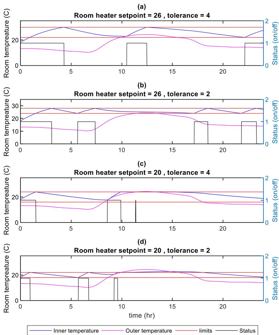
Figure 11: House heater controller output
