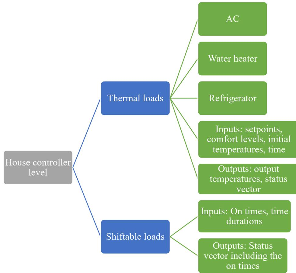
Figure 5: Full house controller model structure
