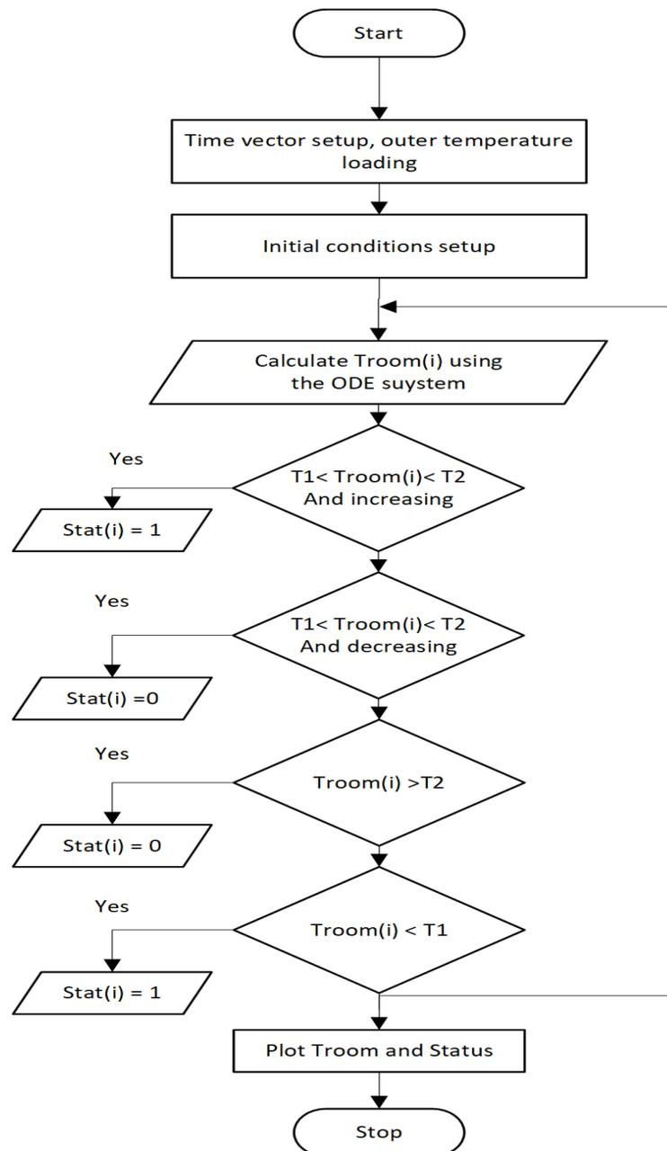
Figure 1: Heating system flowchart
