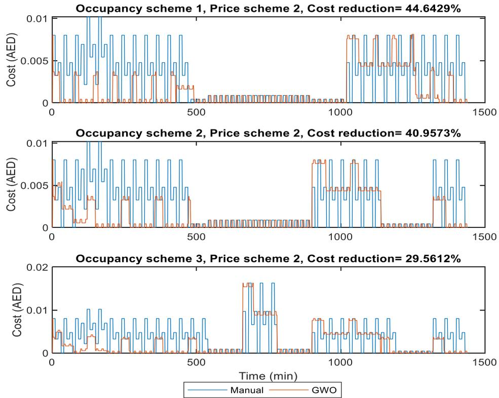
Figure 26: Manual controller cost vs GWO cost for price scheme 2
