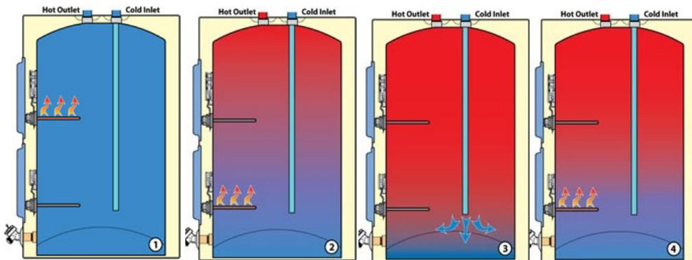
Figure 4: Working cycle of a water heater system
