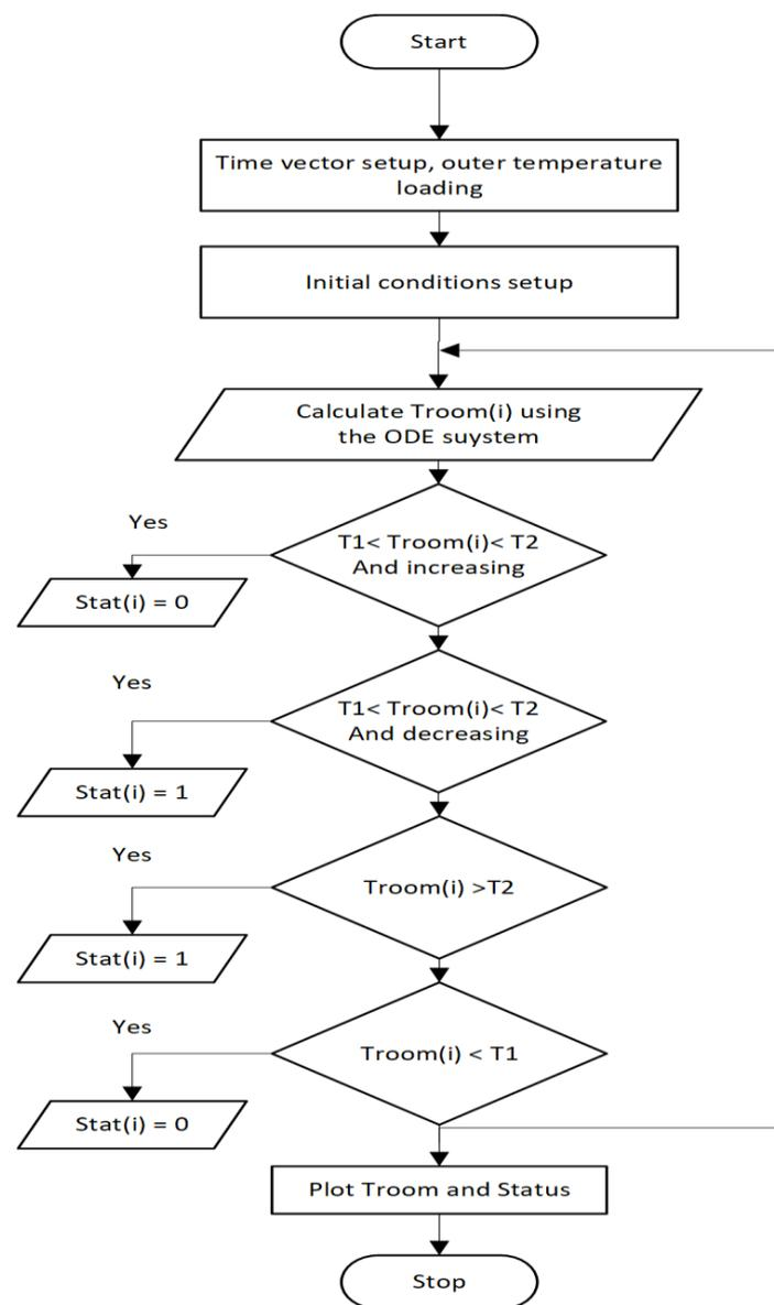
Figure 3: Cooling thermostat system (AC)
