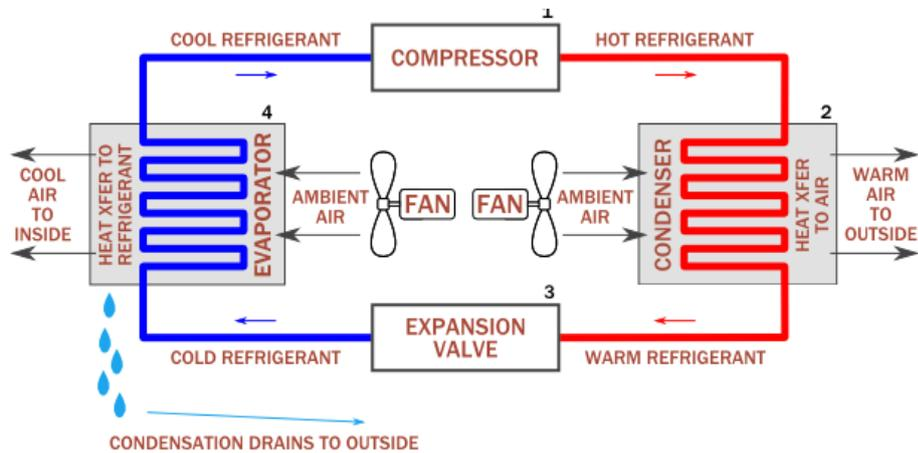
Figure 2: Air conditioner cooling cycle
