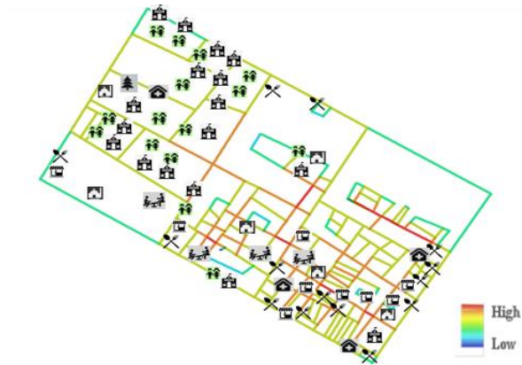
Figure 68: Connectivity Map (Rn) of Al Qusais First, developed by author using DepthmapX
