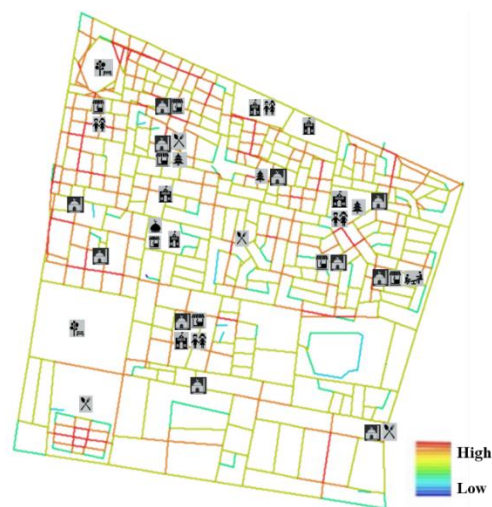
Figure 38: Connectivity Map (Rn) of Al Khawaneej First, developed by author using DepthmapX
