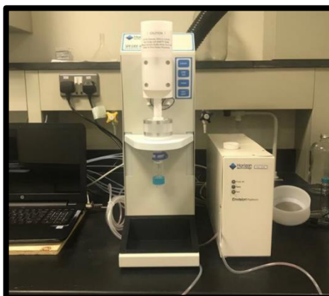
Figure 8: SPE instrument used for purifying wastewater samples
