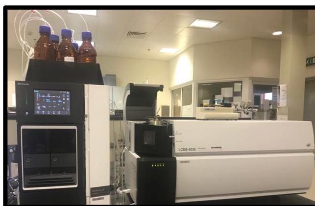
Figure 7: LC-MS/MS used for the analysis of PCs in this study
