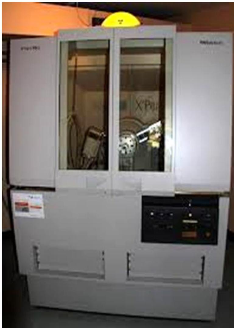
Figure 19: X-ray diffractometer (XRD) and X'Pert PRO system
