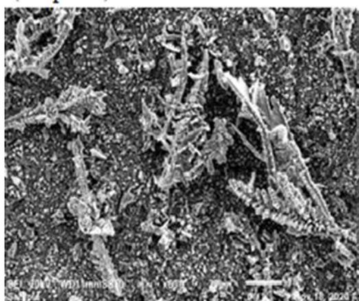
**Zn-Sn solution electrodeposited product
