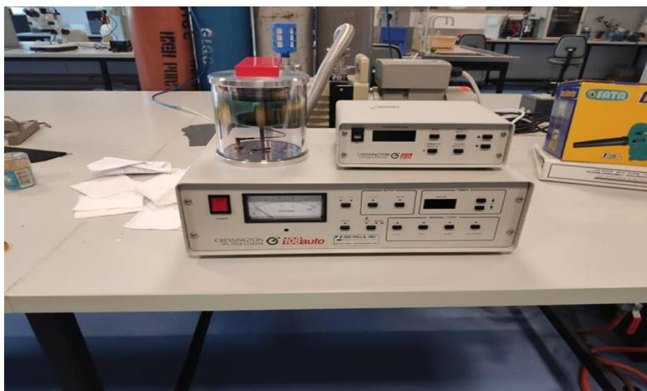
Figure 18: Gold plating device to be used for SEM
