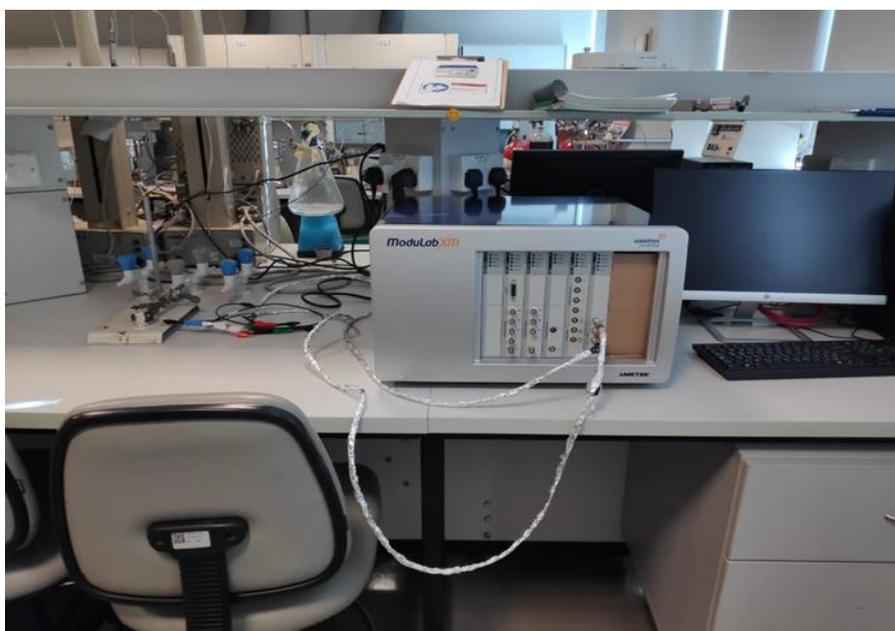
Figure 10: Model Modu-Lab XM ECS- potentiostat - galvanostatic system
