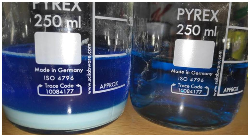
Figure 20: Left jar contains solutions with EDTA; right jar is stable contains sodium citrate
