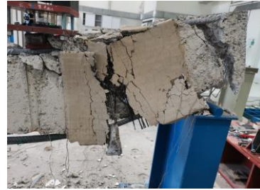
Figure 4.13: Crack pattern of specimen NS-G1-90: A. Picture of the beam at failure, B. Close views at failure (east shear span)
