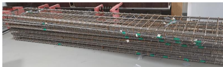
Figure 3.5: Steel cages of the beams with stirrups
