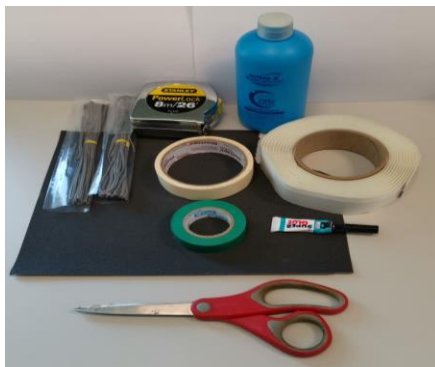
Figure 3.10: Installation of strain gauges: A. Materials used, B. Bonding strain gauges to steel bars
