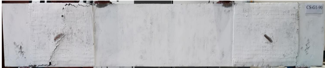
Figure 4.13: Crack pattern of specimen NS-G1-90: A. Picture of the beam at failure, B. Close views at failure (east shear span)
