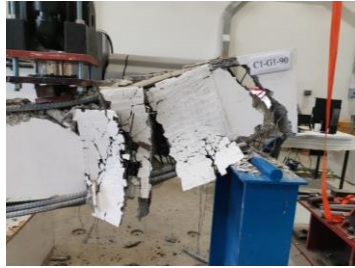
Figure 4.13: Crack pattern of specimen NS-G1-90: A. Picture of the beam at failure, B. Close views at failure (east shear span)
