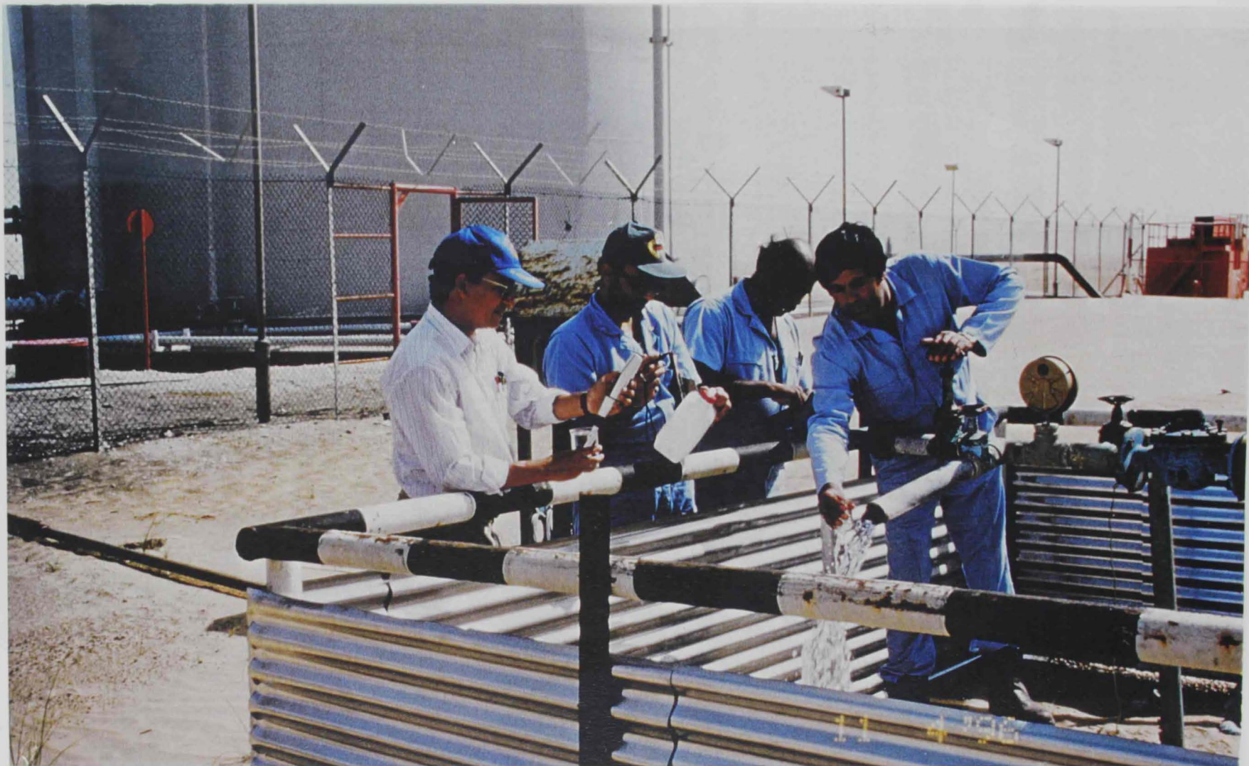
Figure 29. Water sampling and measurement of temperature, pH and electrical conductivity in a domestic water well of the Bu Hasa Field in April 1996.
