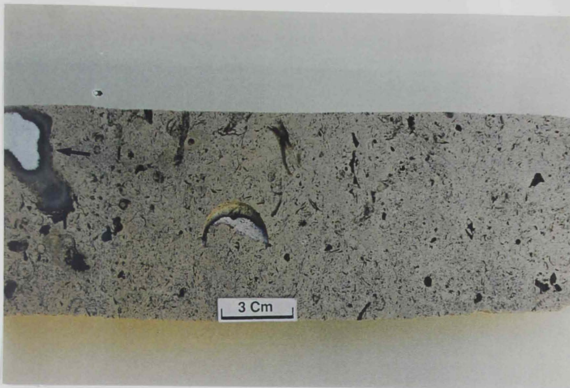
Figure 15. Core photograph (depth= 771ft.) of light gray to light brown, black spotted bioclastic limestone (wackestone-packstone), with some gypsum nodules (arrow).
