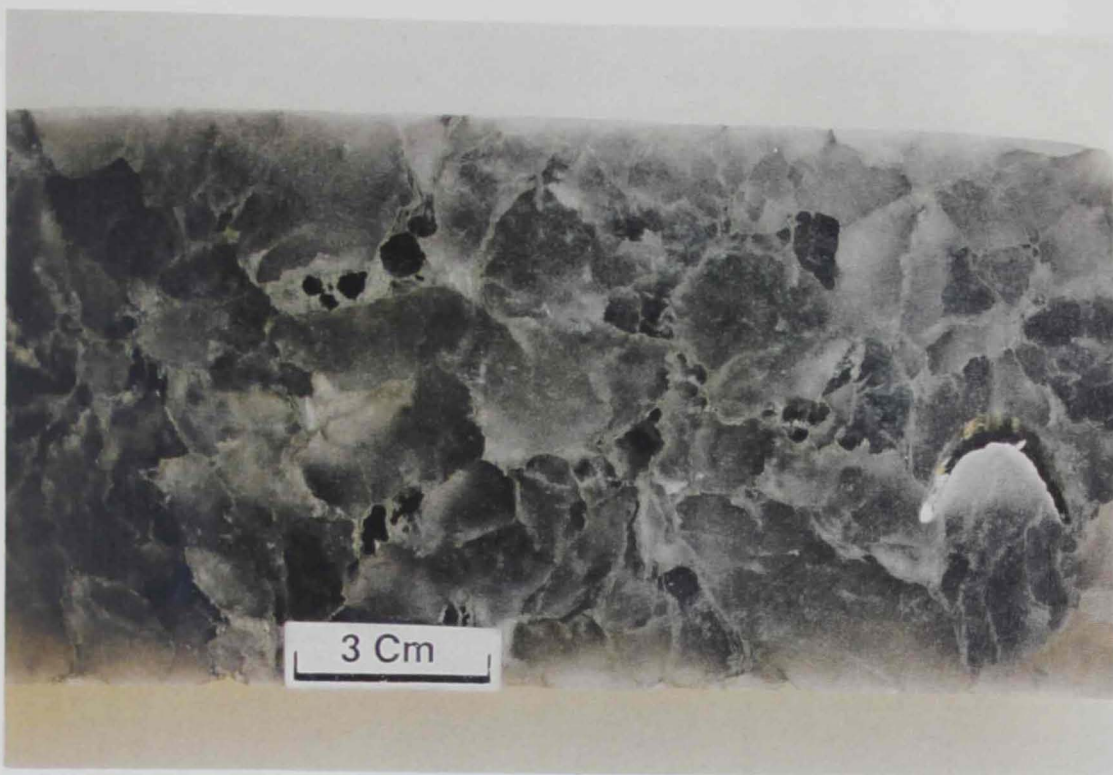
Figure 17. Core photograph (depth = 781ft. and 4 in) showing an interval of dark gray gypsum with cloudy appearance.
