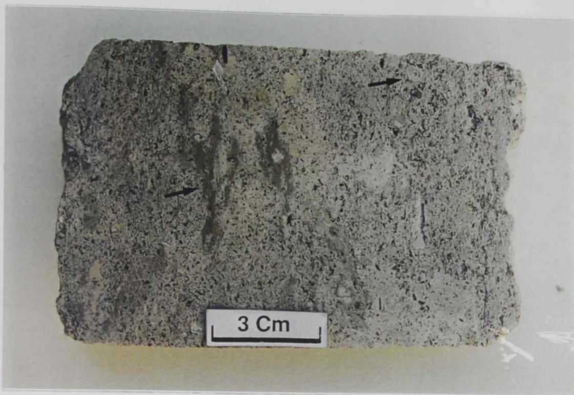
Figure 13. Core photograph (depth = 709ft. and 7 in) of gray, whitish gray limestone (wackestone-packstone) with clay clasts and large well-preserved echinoids fragments (arrows). Notice the relatively high porosity due to leaching.
