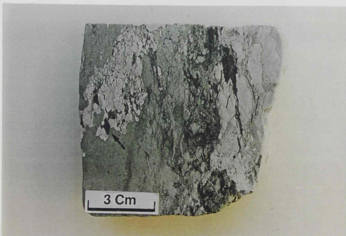
Figure 16. Core photograph (depth=778ft. and 10 in) of mudstone-siltstone of greenish to light gray color. The rock is locally nodular with fine dark clayey material (arrow).
