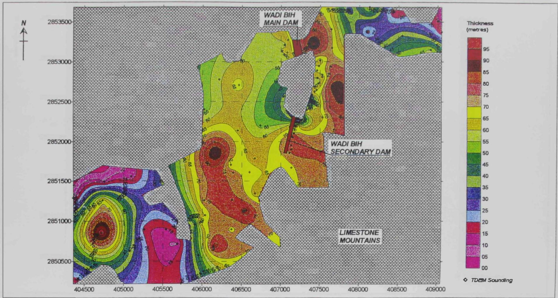
Fig. (3.9) Thickness distribution map of the third layer
