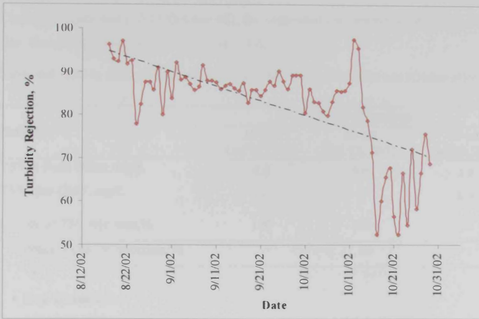
Figure 4-13: Degree of turbidity rejection (Ondeo pilot plant)
