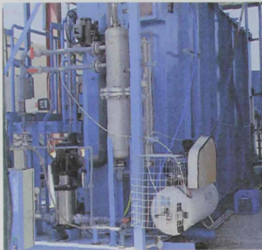
Figure 4-9: Flotation system (Ondeo pilot plant)
