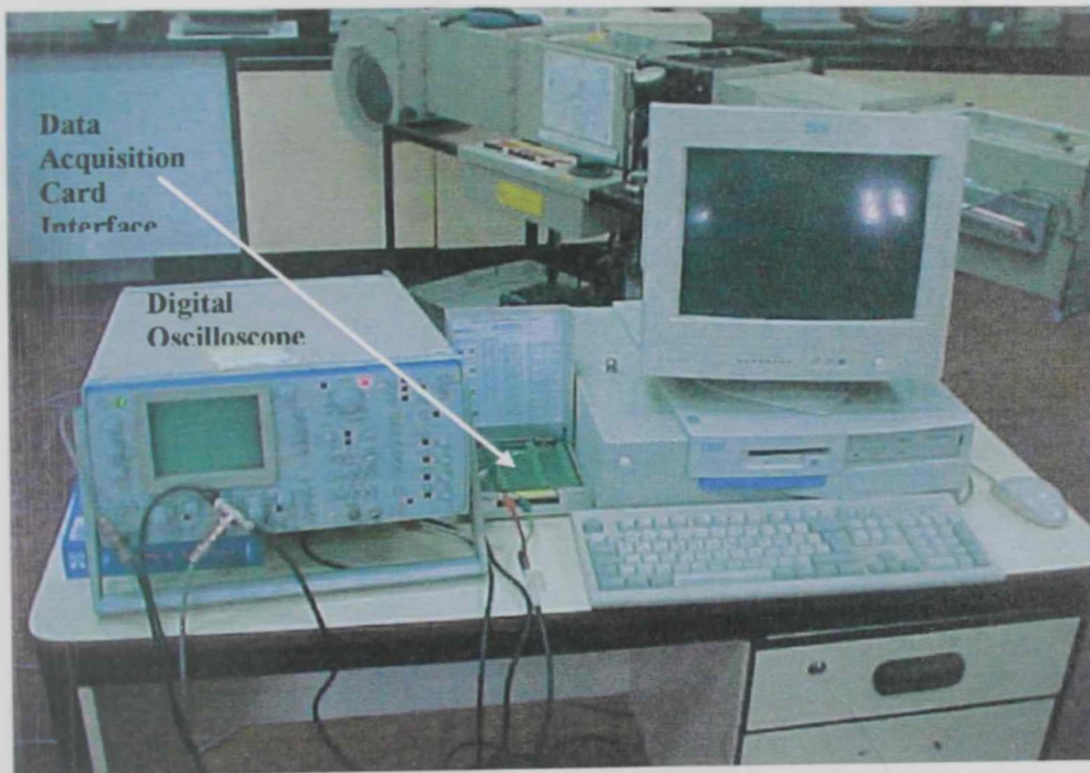
Figure 3.15. Photo of the DAS Cards and connections to sensors
