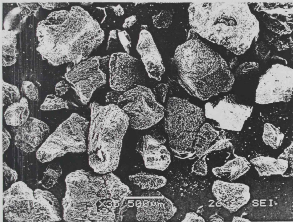
Figure 4-1 Scanning electron microscope picture of PDKAC units (peds) and the macropores.
