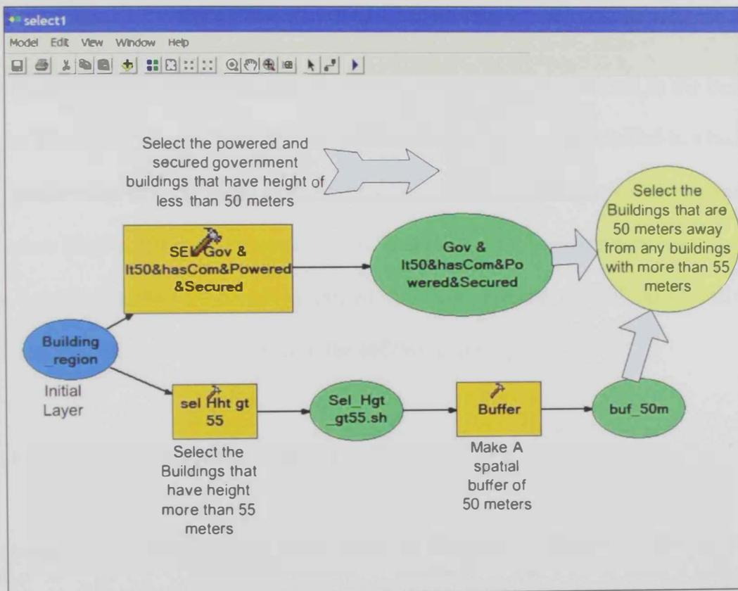
Fig. 6.4 Spatial Analysis Model (Using ESRI Model Builder 9.1)
