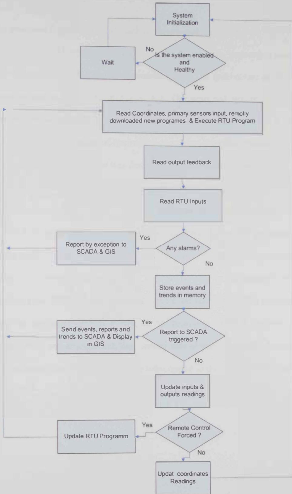
Fig. 8.2 Flow chart for the RTK Network & SCADA/GIS Logic control
