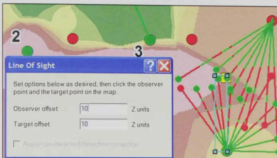
**Fig. 7.3 Examining the line of sight between stations according to the observer and target heights from ground**
