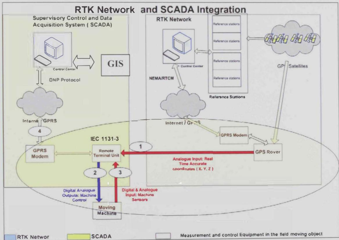
Fig. 8.1 Proposed RTK reference network & SCADA integration
