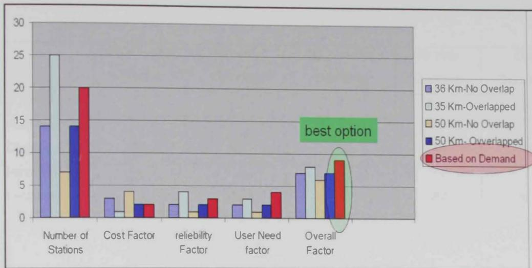
**Fig. 5.6 Station distribution options with their weighing factors**
