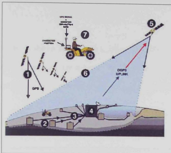
Fig. 3.2 SBAS Service Exemple : Omni STAR SBAS service
