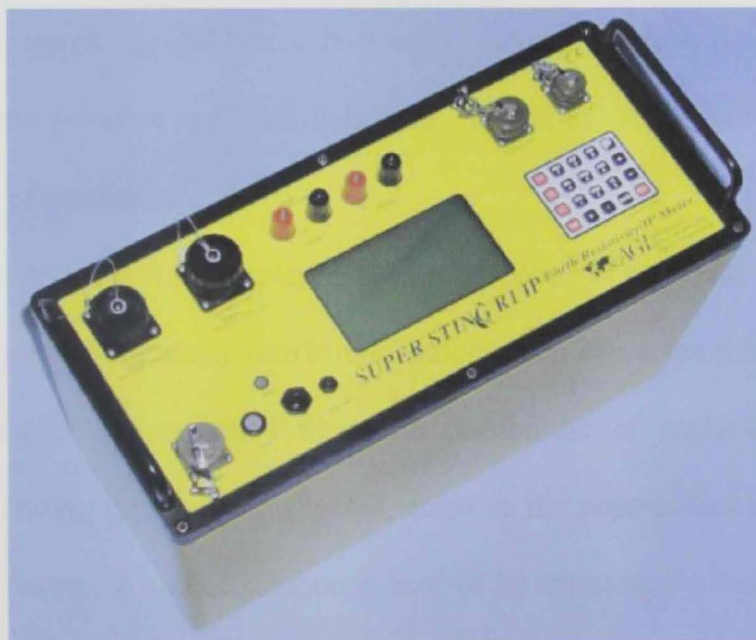
Figure 3.5. Single Channel Memory Resistivity and IP meter.
