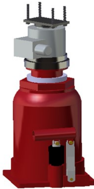
Figure 25: 3D model of load cell and hydraulic jack
