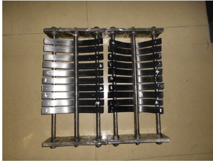
Figure 12: Bending fixture for CFRP plates. (Kafodya et al., 2015)
