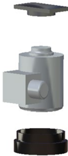
Figure 24: Model of load cell and it's mounting
