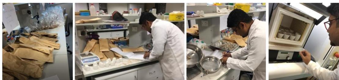
Figure 14: Lab works, preparing samples, grinding, weighing, and drying.
