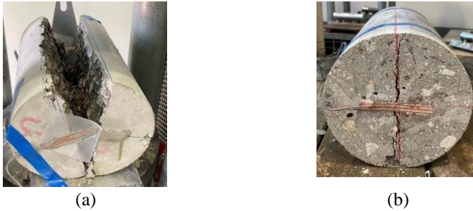
Figure 2.29: Failure modes of concrete cylinders under splitting tensile tests: (a) R0-SF0, (b) R100-SF1
