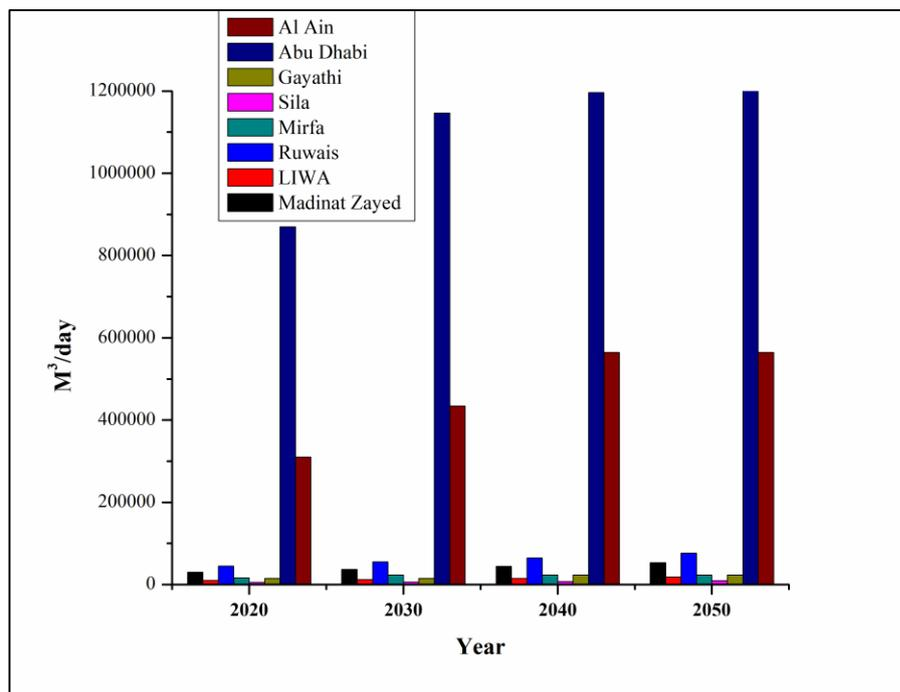
Figure 17: Capacity expansion for the TS plants at all locations
