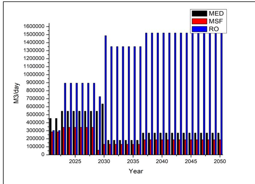
(e) Capacity required for different years at Fujairah
