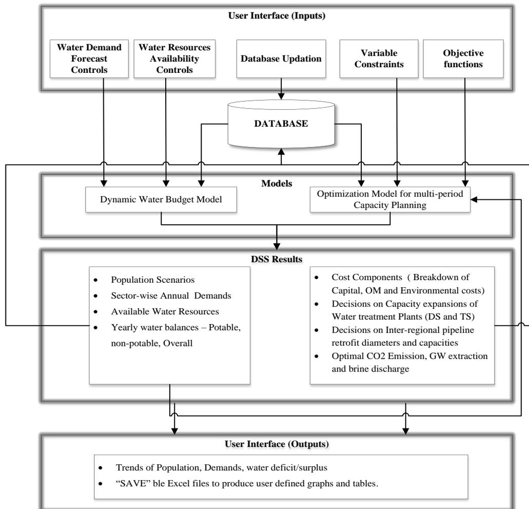
Figure 21: Conceptual Design of the SuWaB-AD Decision Support Tool
