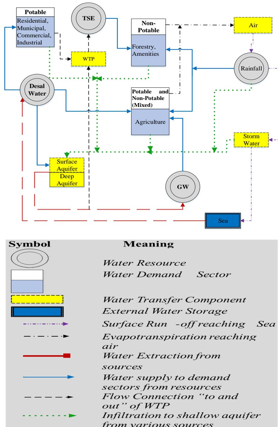
Figure 3: Schematic representation of water system of Abu Dhabi.
