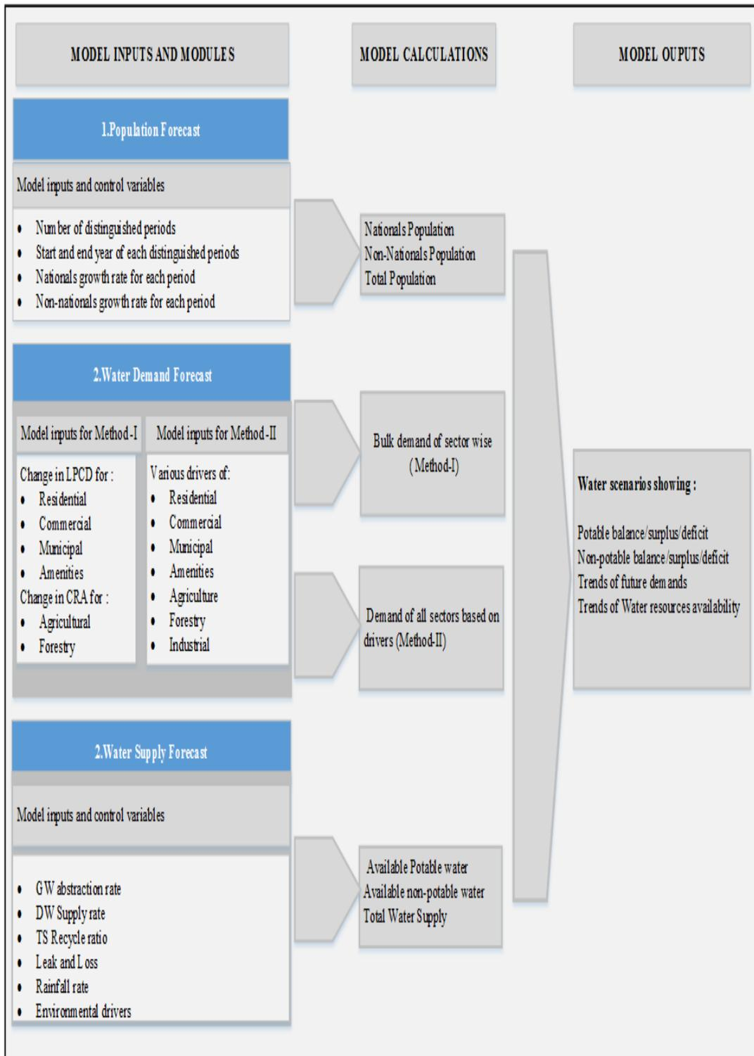
Figure 4: Schematic representation of dynamic model (ADWBM)
