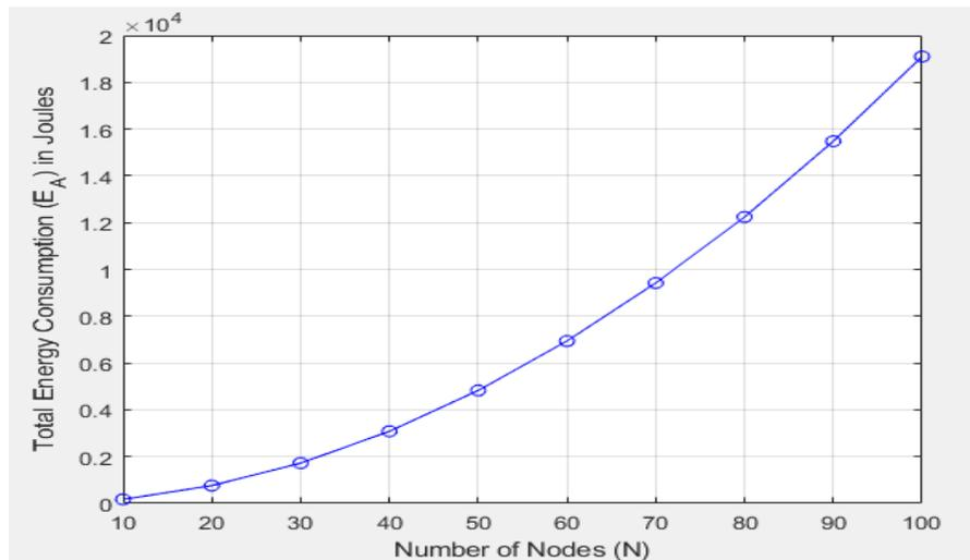
*Figure 8 Variation of Energy Consumption with Number of Nodes using broadcast-based protocols*
