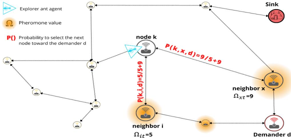
Figure 4 The process of selecting the next hope to the demander node
