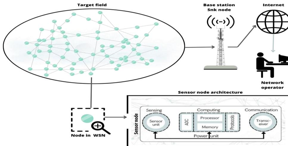
Figure 1 Wireless sensor network (WSN)
