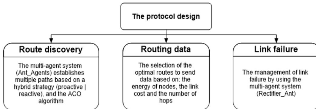
Figure 2 The components of the proposed protocol
