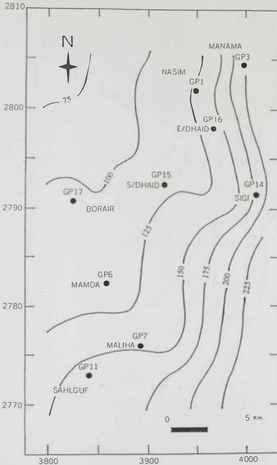
Figure 4.5 Hydraulic head contour map of the upper aquifer in the Al Dhaid area, in meters above sea level, in 1999.
