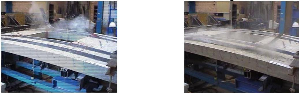
Figure 2.3: Debonding of CFRP (Kim and Smith 2009)
