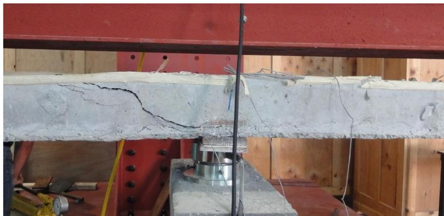
Figure 4.25: Photo of specimen B-S2-H4 at failure
