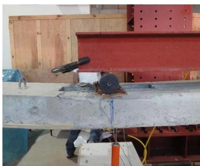
Failure of mid-span section
