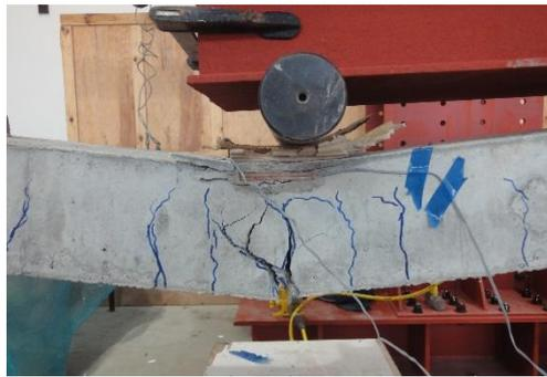
Failure of mid-span section
