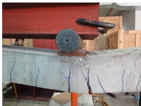
Failure of mid-span section
