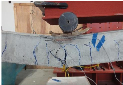
Failure of mid-span section
