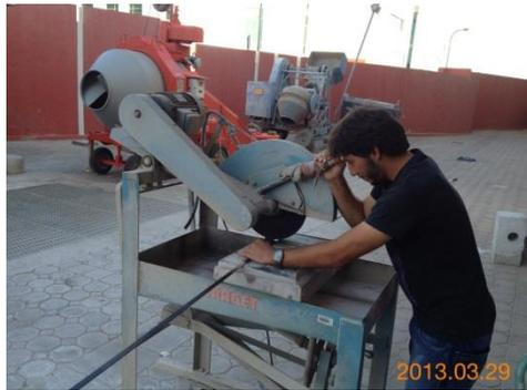
(a) Cutting of CFRP strips
