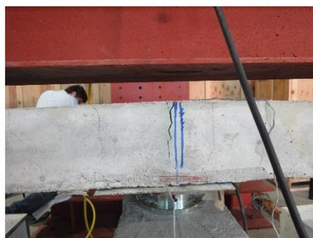
Failure of section over central support
