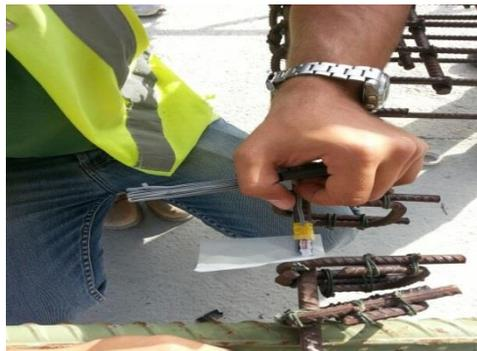
(c) Bonding of S.G. to steel surface
