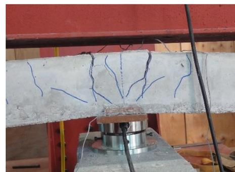
Failure of section over central support
