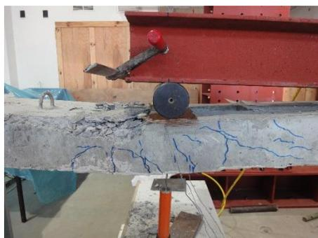
Failure of mid-span section
