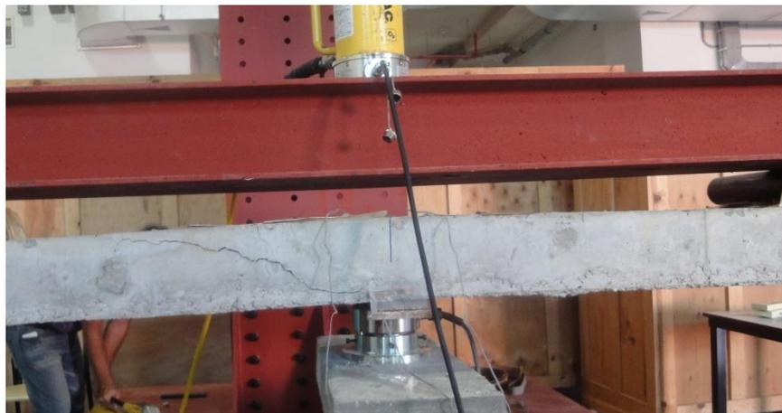
Figure 4.24: Photo of specimen B-S2-H2 at failure
