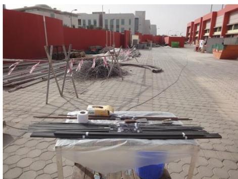
(a) CFRP strips (Sika® Carbo Dur)
