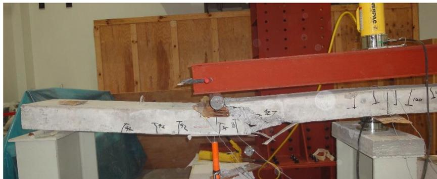
Figure 4.3: Photo of specimen A-S2-H0 at failure
