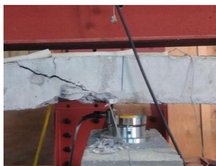
Failure of section over central support
