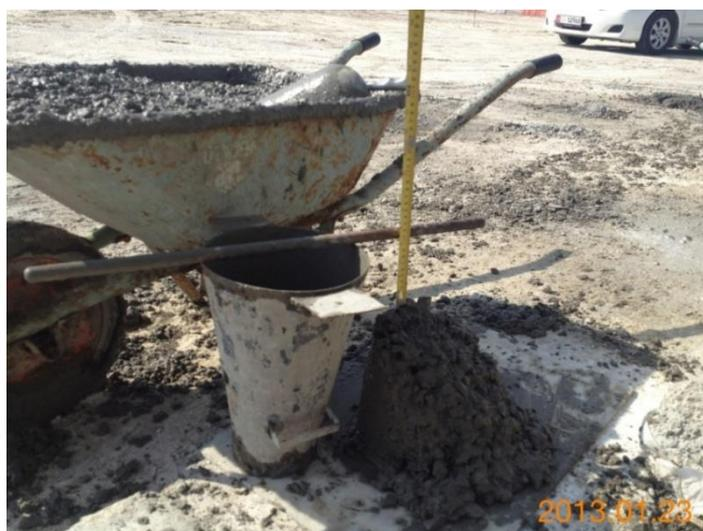
Figure 3.13: Slump test
