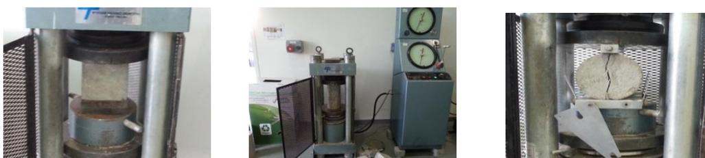
(a) Cube compression test    (b) Cylinder compression test    (c) Cylinder splitting test
