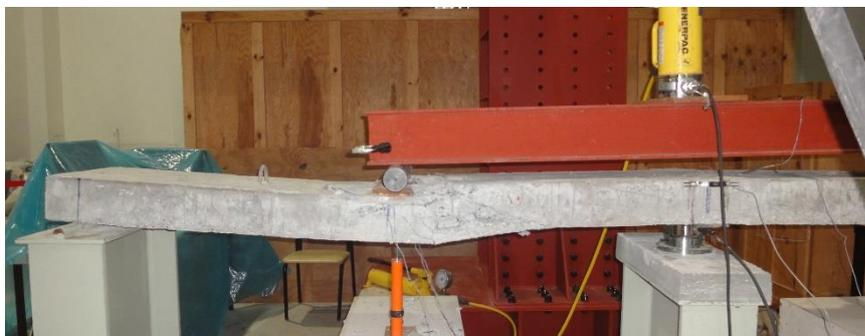
Figure 4.6: Photo of specimen A-S4-H2 at failure
