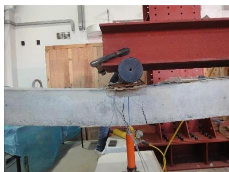
Failure of mid-span section
