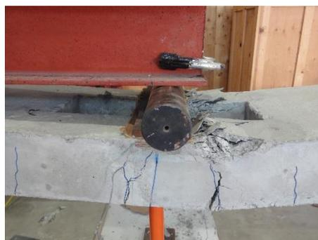
Failure of mid-span section
