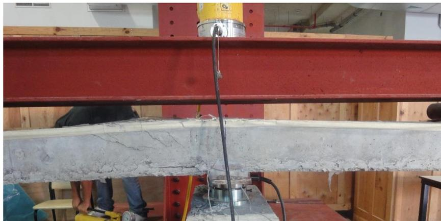
Figure 4.23: Photo of specimen B-S0-H4 at failure
