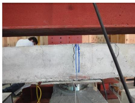
Failure of section over central support
