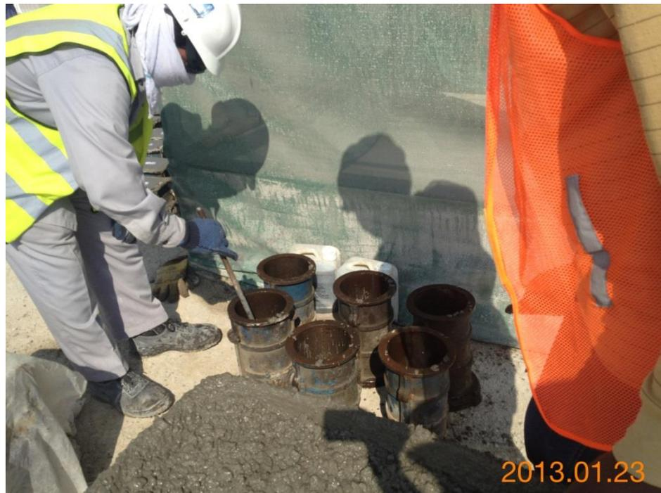
Figure 3.9: Preparation of concrete cylinder samples
