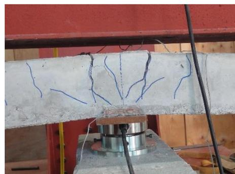
Failure of section over central support
