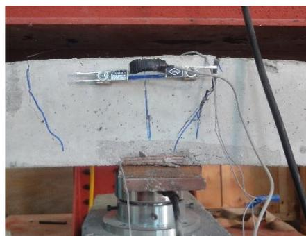
Failure of section over central support
