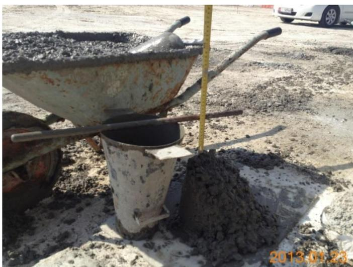
Figure 3.13: Slump test
