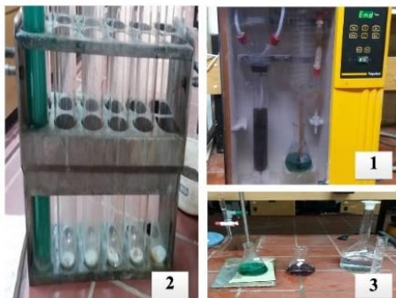
Figure 2. Protein measurement, (1) digestion, (2) distillation, and (3) titration
