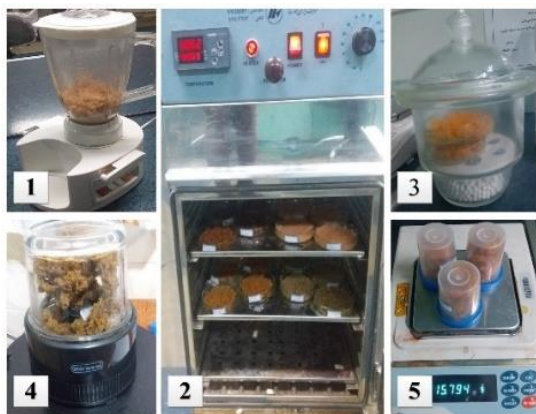
Figure 1. Dry matter measurement: (1) mixing, (2) drying in the oven, (3) placing in a desiccator, (4) grinding, (5) weighing the dry sample
