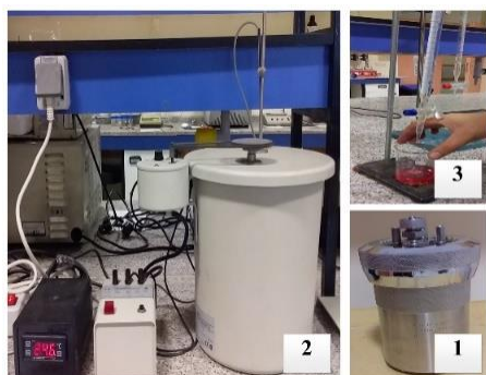
Figure 4. Energy measuring using a calorimeter bomb: (1) Combustion chamber, (2) Calorimeter
