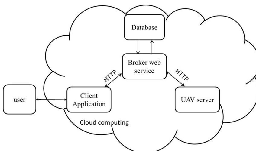
Figure 4-4 Client-Server Architecture with broker layer.
