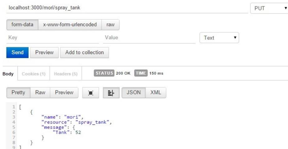
Figure 5-10 Reading the remaining tank capacity of the spraying service UAV
