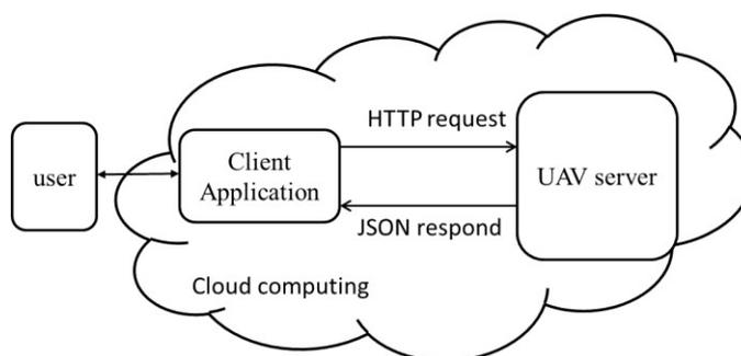
Figure 4-1 Client-Server Architecture.
