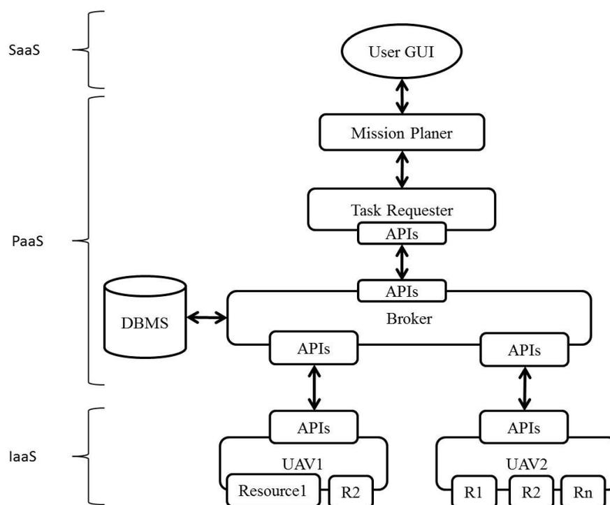
Figure 3-1 UAV-Cloud Framework
