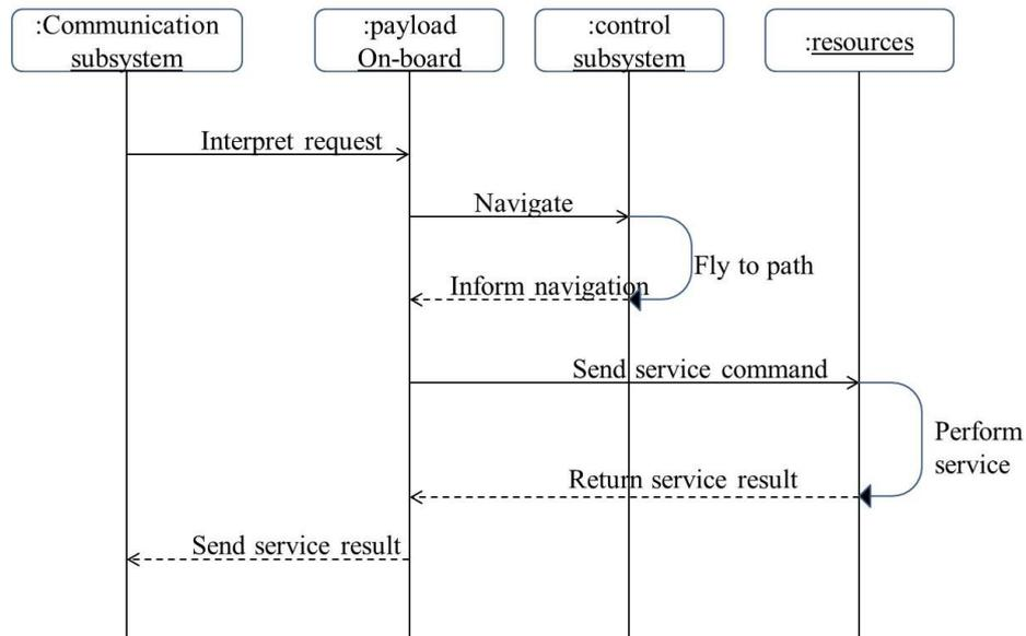
Figure 3-2 Service request sequence diagram for UAV subsystems.
