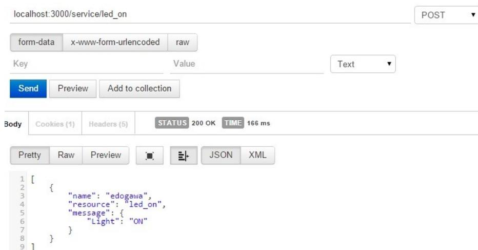
Figure 5-7 *POST* operation request and response for 'led\_on' service through the broker.
