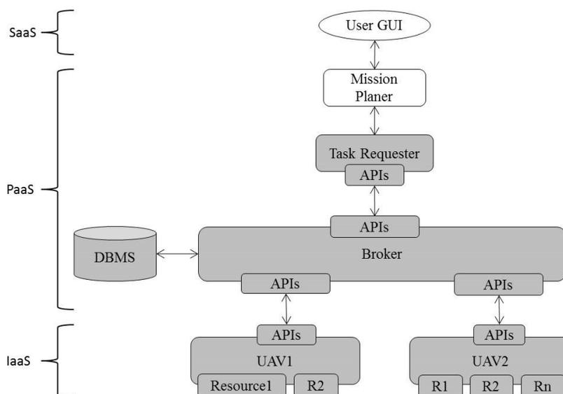
Figure 5-1 The implemented system components of the UAV-Cloud architecture are shaded in gray.
