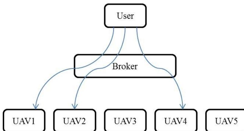
Figure 4-3 Broker layer to separate the application layer from the UAV layer.
