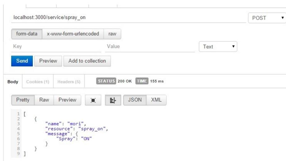
Figure 5-6 *POST* operation request and response for spraying service through the broker
