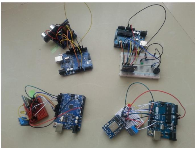
Figure 5-2 Four Arduino boards connected with Adafruit CC3000 boards as well as sensors and actuators representing UAV payload systems and their resources.
