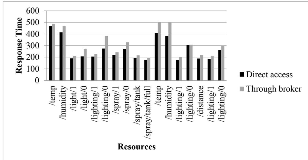
Figure 5-13 Response times of UAV resources with direct accesses and through the broker.
