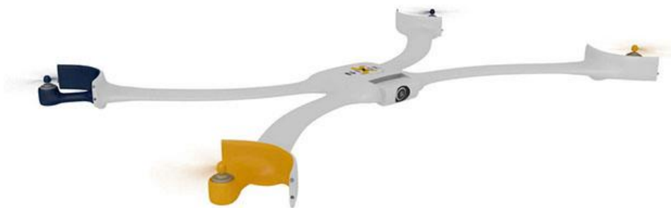
Figure 3-5: Nixie, a wearable UAV (Dent, 2015)
