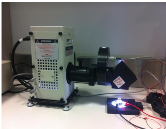
Figure 3.13 The cell under the solar simulator illumination.
