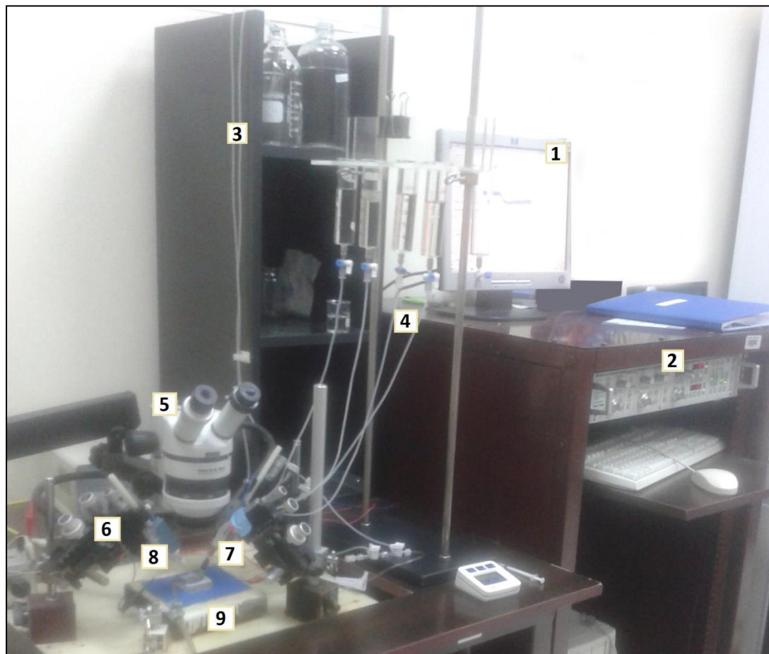
Figure 3.2: A photograph of the two-electrode voltage clamp used to study the alpha7 nicotinic receptor in Xenopus oocyte. ACh solution (4,7) and perfusion solution (3) lines are connected by tubes to the chamber (9). Micromanipulators (6) are used to control electrodes (8) to impale the oocyte visualized using microscope (5). An amplifier (2) is used to record current traces (1); Acquired data were stored on a computer (Prof. Murat Oz Lab).
