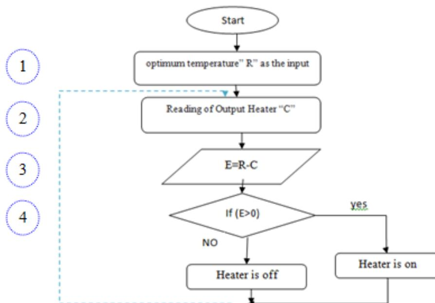
Figure6. Flowchart of algorithm implemented by the controller
