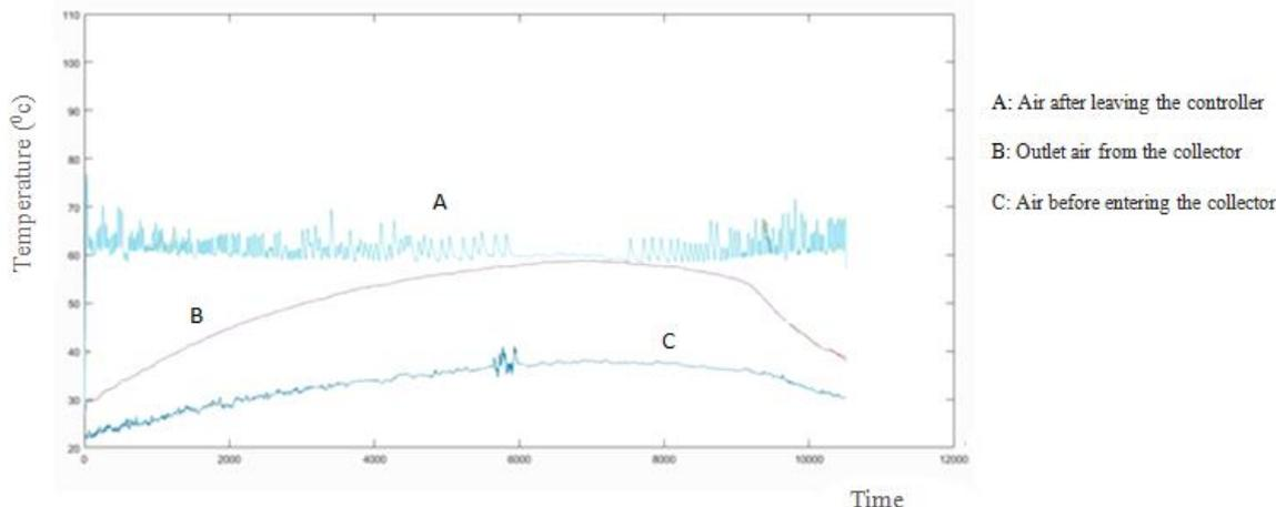
Figure9. Performance of the controller in the event that the three elements simultaneously turn on and off
