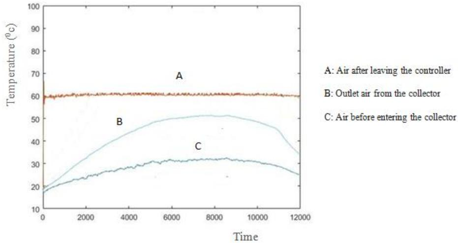
Figure7. Performance of temperature controller at 60 ° C in sunny day
