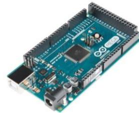
Figure4. Microcontroller board (Model: Mega2560 R3)
