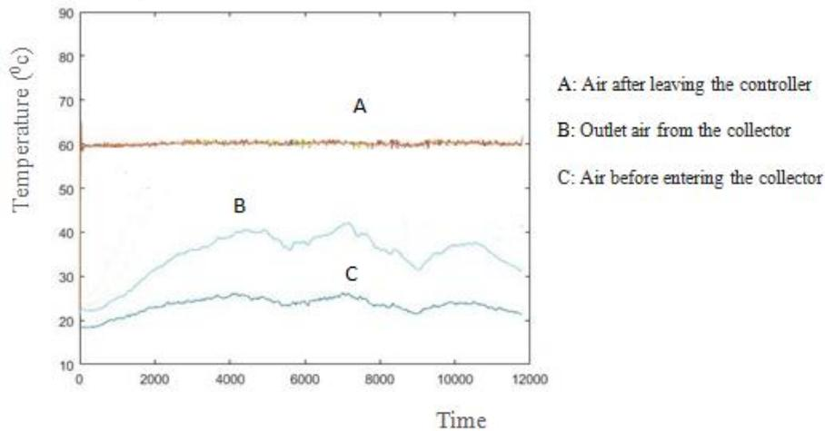
Figure8. Performance results of control at 60 ° C in semi-cloudy day with strong wind
