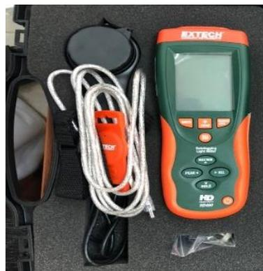
Fig. 4. Light metre used for measuring daylighting (0 lux–400 Klux).
