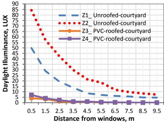
Fig. 6. Average daylight penetration (lux) into four classrooms.
