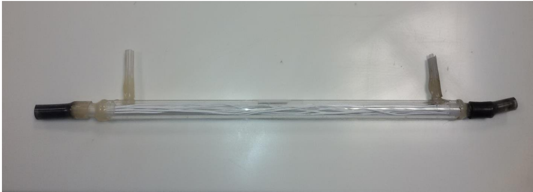
Figure 6: A real PVDF hollow fibers membrane contactor module constructed in the lab
