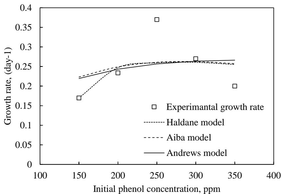
Figure 26: Growth rates of microalgae at different phenol concentrations *Tetraselmis* sp.
