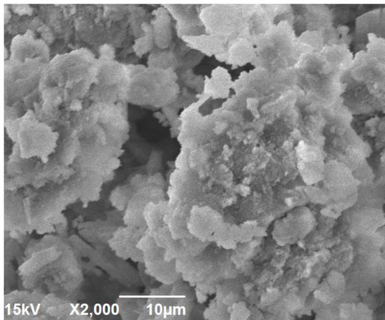
Figure 31: Catalyst morphology before calcination
