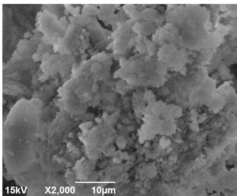
Figure 32: Catalyst morphology after calcination
