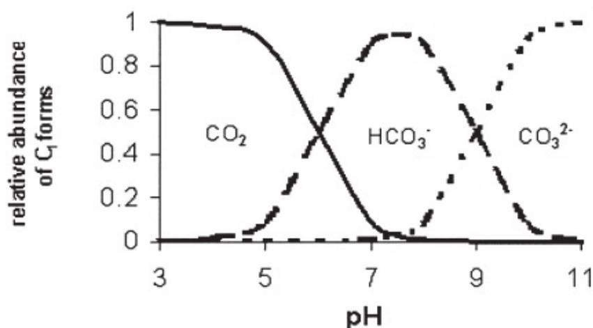
Figure 5: Effect of changing pH on the relative abundance of carbon forms
