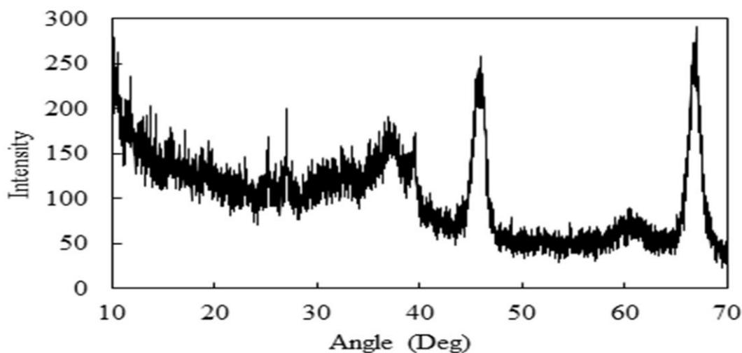
Figure 33: Catalyst intensity before calcination
