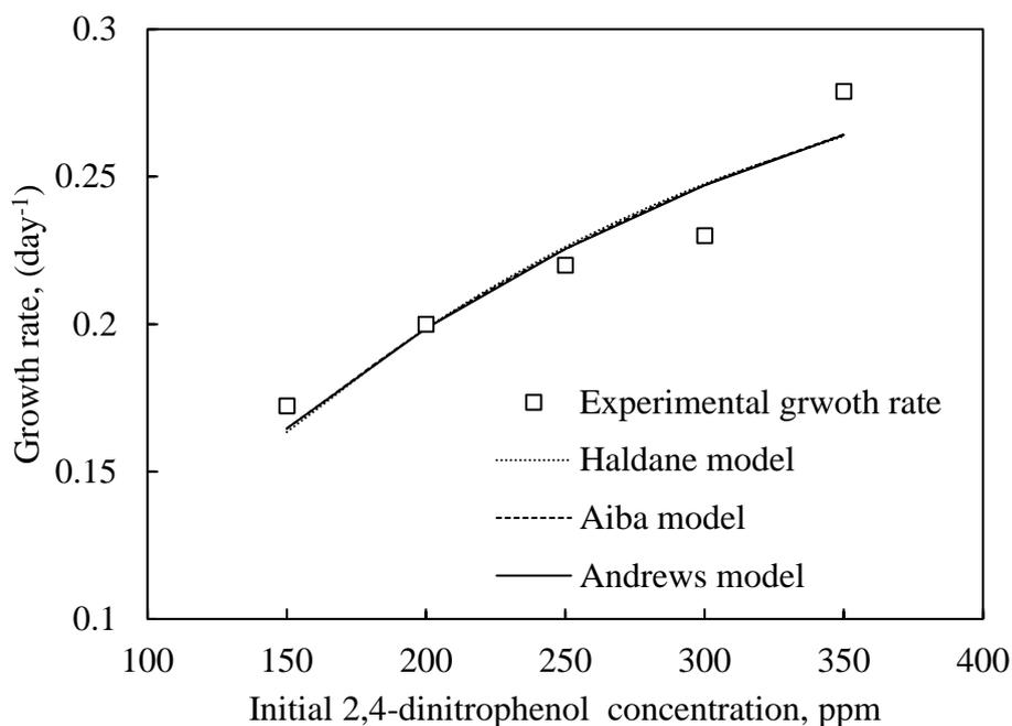
Figure 30: Growth rates of microalgae at different 2,4-dinitrophenol concentrations using *Tetraselmis sp.*
