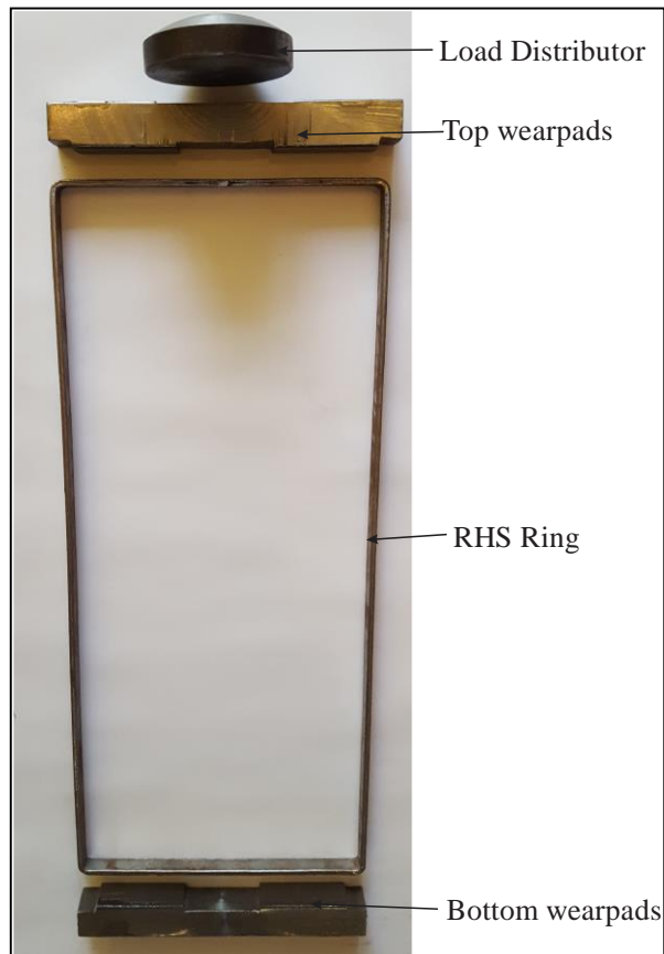
Figure 52: Assembly of RHS ring between wearpads
