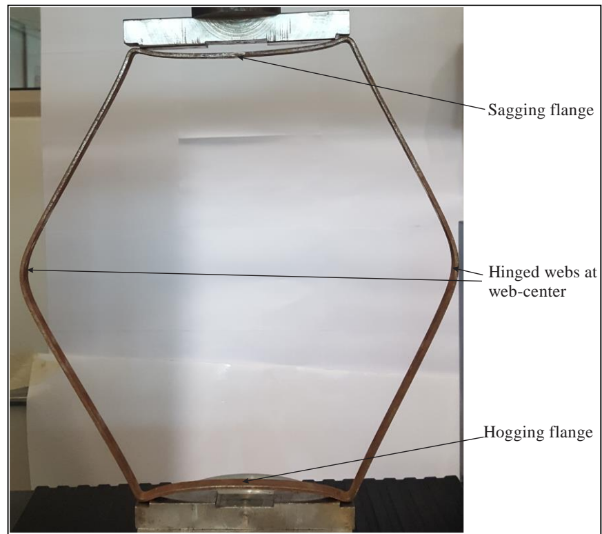
Figure 57: Hinged webs at web center and bent flanges due to compression between wearpads
