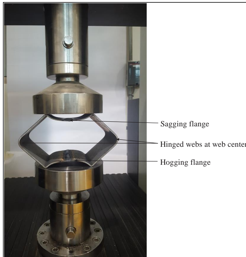
Figure 64: RHS piece with hinged webs and bent flanges between platens
