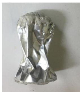
Figure 18: Irregular sample foamed at 0 LBS packing pressure
