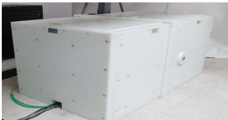
Figure 2: Moderated & Shielded DD109.4 Neutrons-Generator at University of Sharjah [21]
